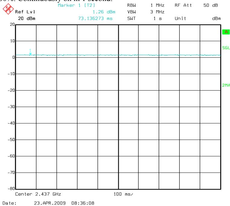
802.11b Duty Cycle 100%: Continuously on for most of 1 second:
