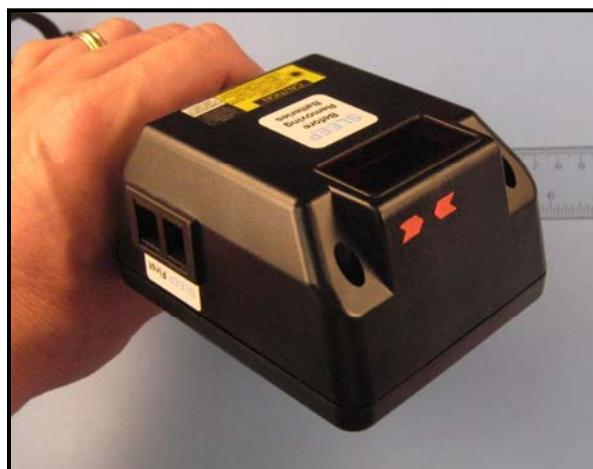
The antenna is located approximately 9 cm from the nearest finger as shown in the below photograph. The red paper in the photograph is 5 cm square.
