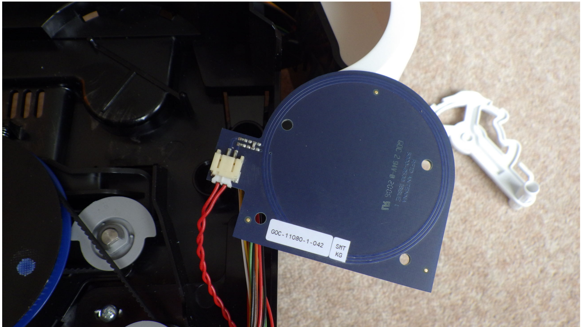
RFID antenna close-up (lifted from mounting position and turned to show detail)
