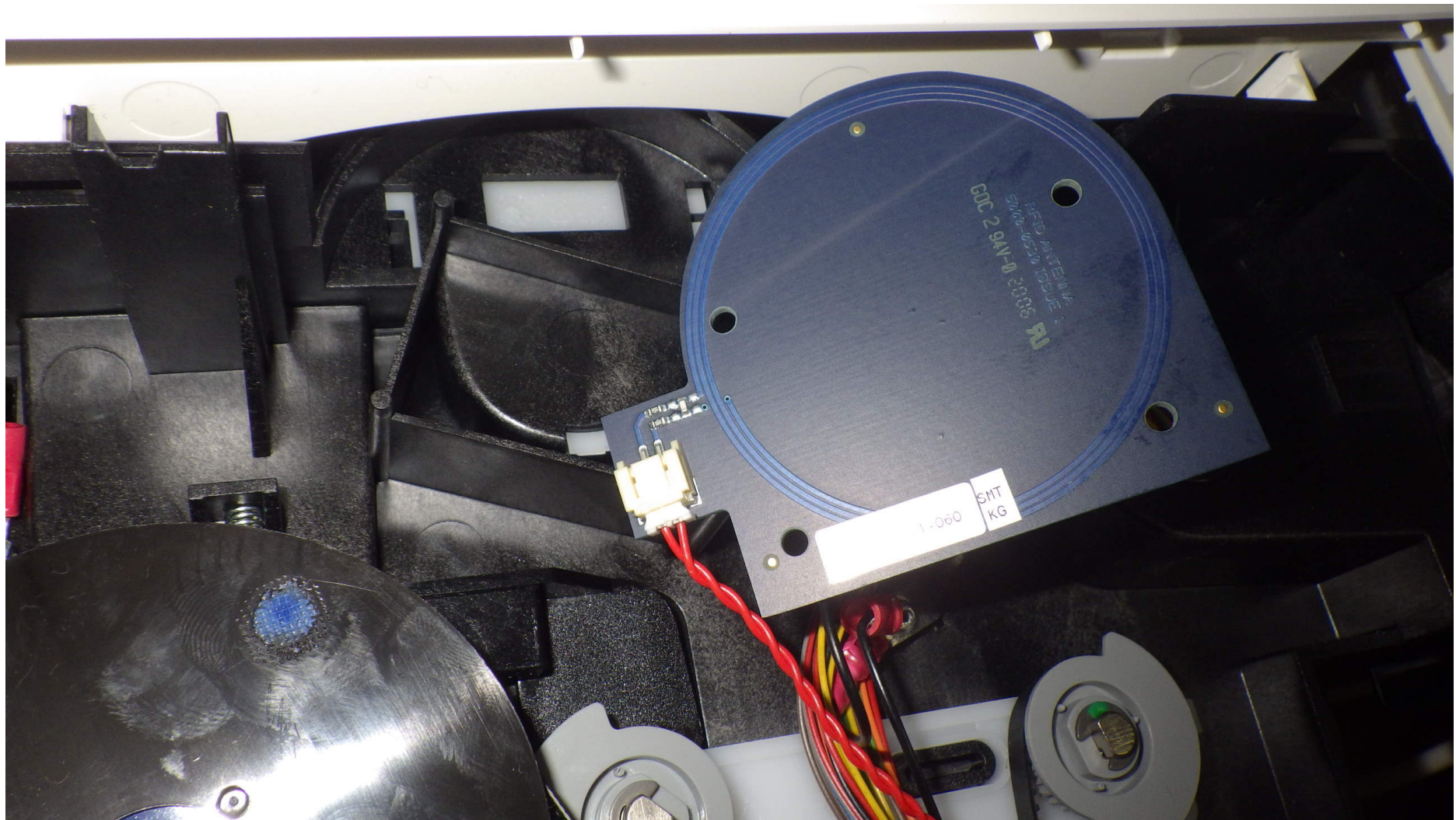
Magicard RFID antenna close-up (lifted from mounting position and turned to show detail)
