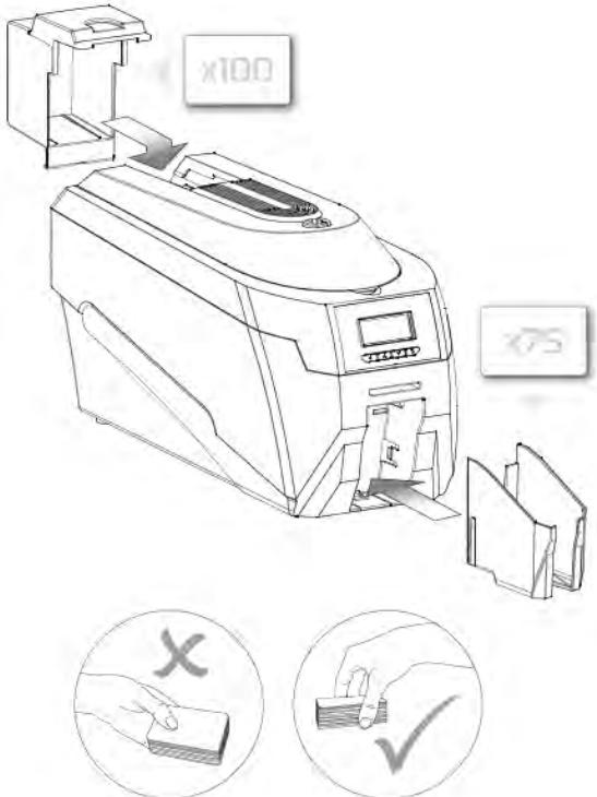
**HOPPER:** Insert the hopper into the aperture at the back of the printer and click into place.
