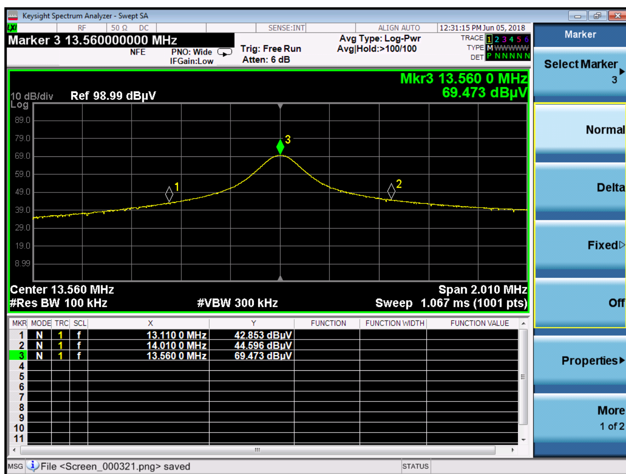
Figure 13: Band Edge Measurement – conducted test
