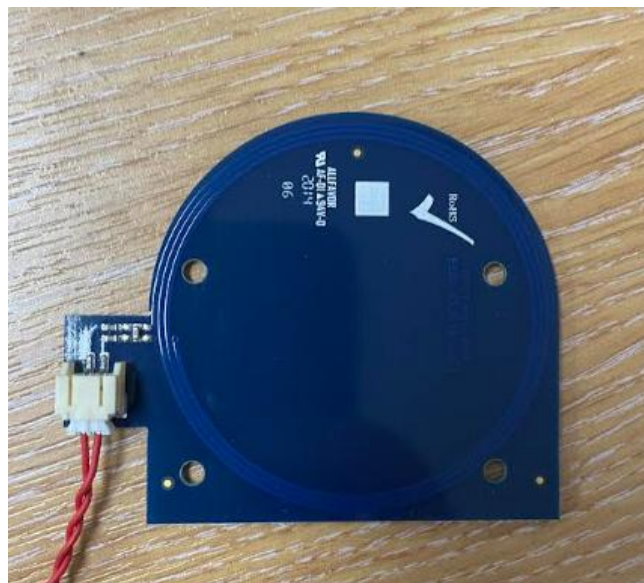
Figure 8: View of RFID Antenna removed from the product
