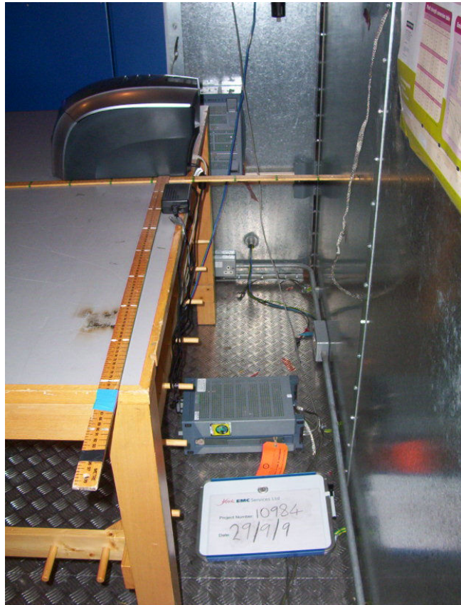
Photograph 5.7.1 Conducted emissions testing
