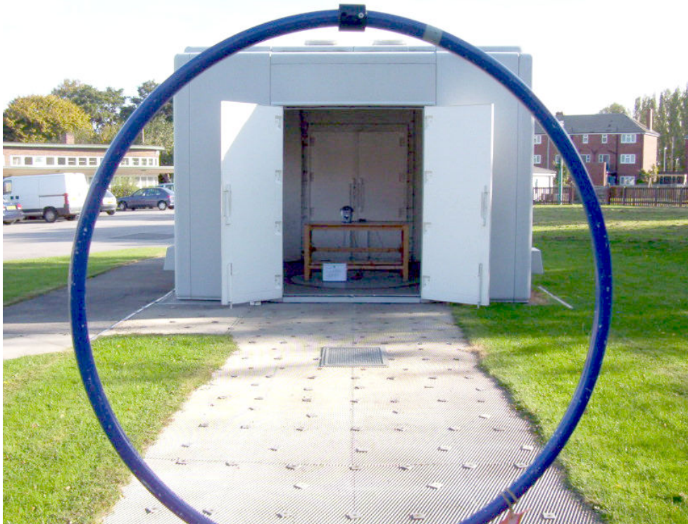
Photograph 5.7.3 Radiated emissions testing (9kHz to 30MHz), Open Area Test Site
