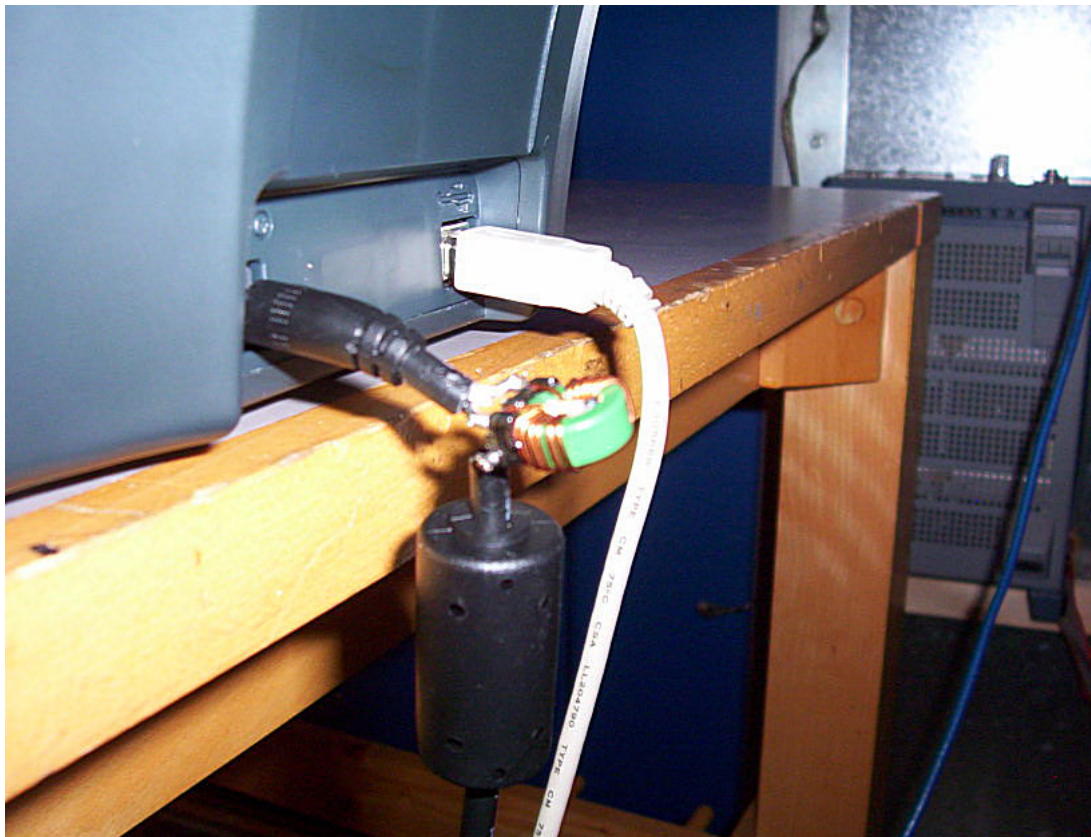
Fig 5.10.1, 30uH common mode choke fitted to mains supply lead
