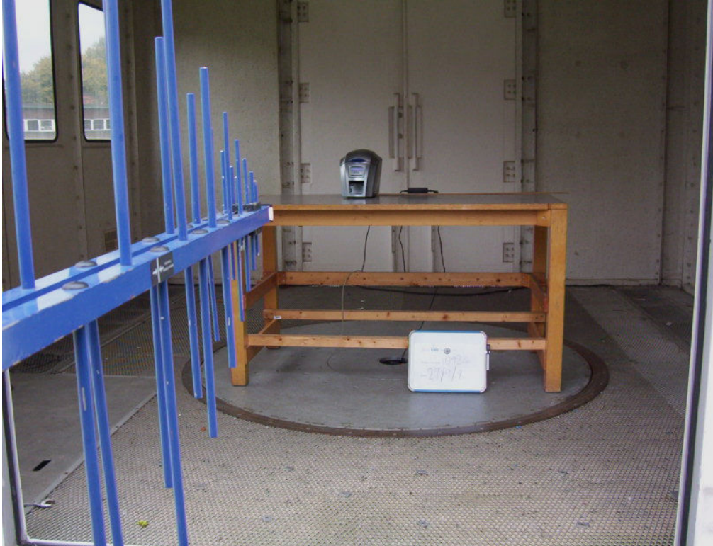
Photograph 5.7.3 Radiated emissions testing (30MHz to 1GHz), Open Area Test Site
