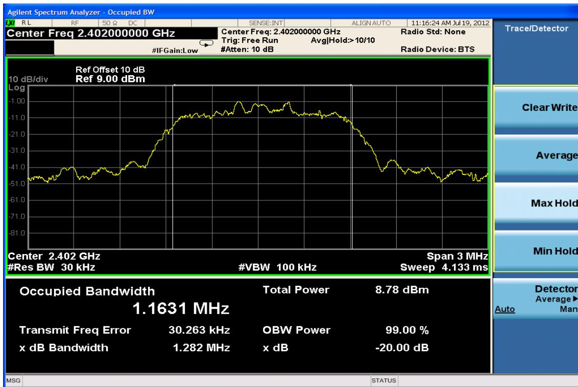
**99% & 20dB Bandwidth Test Data CH-Mid**
