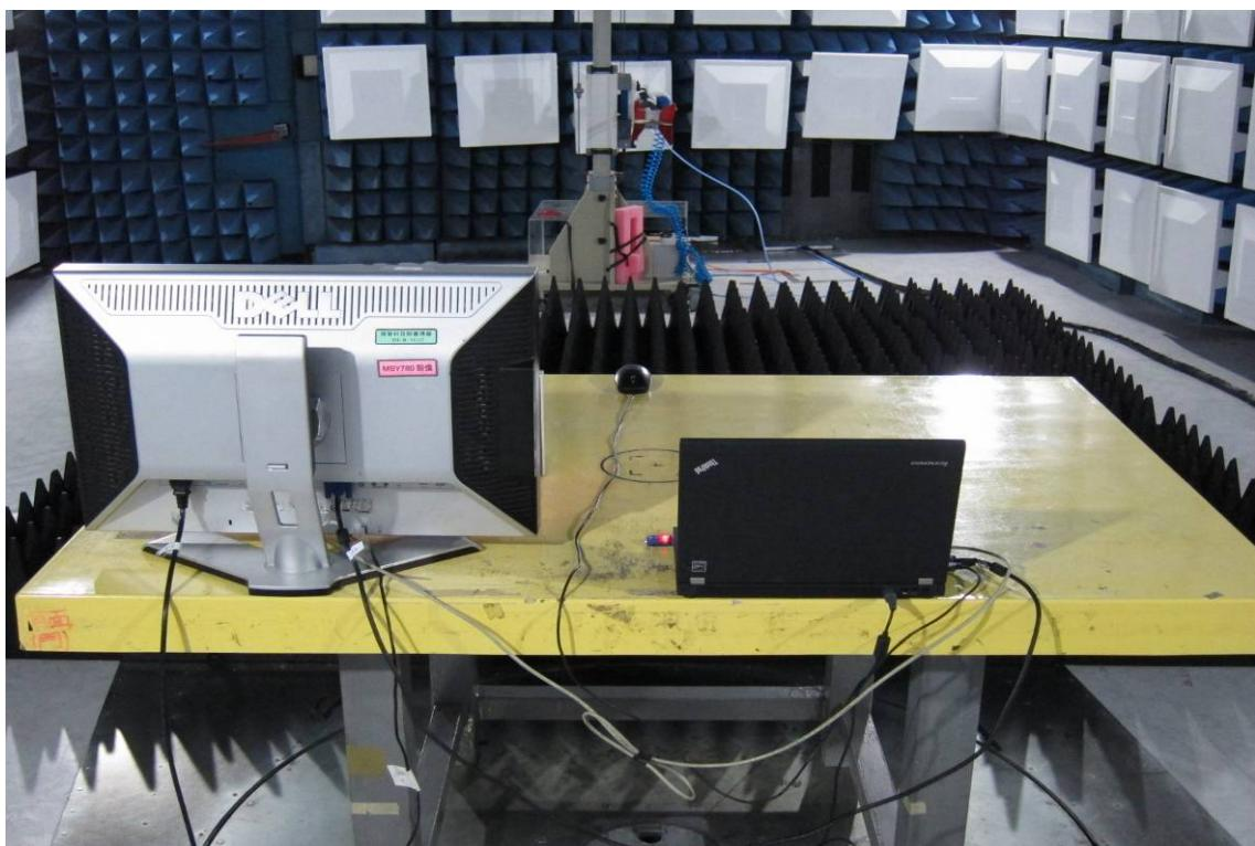
**AC POWER LINE CONDUCTED EMISSION TEST**
