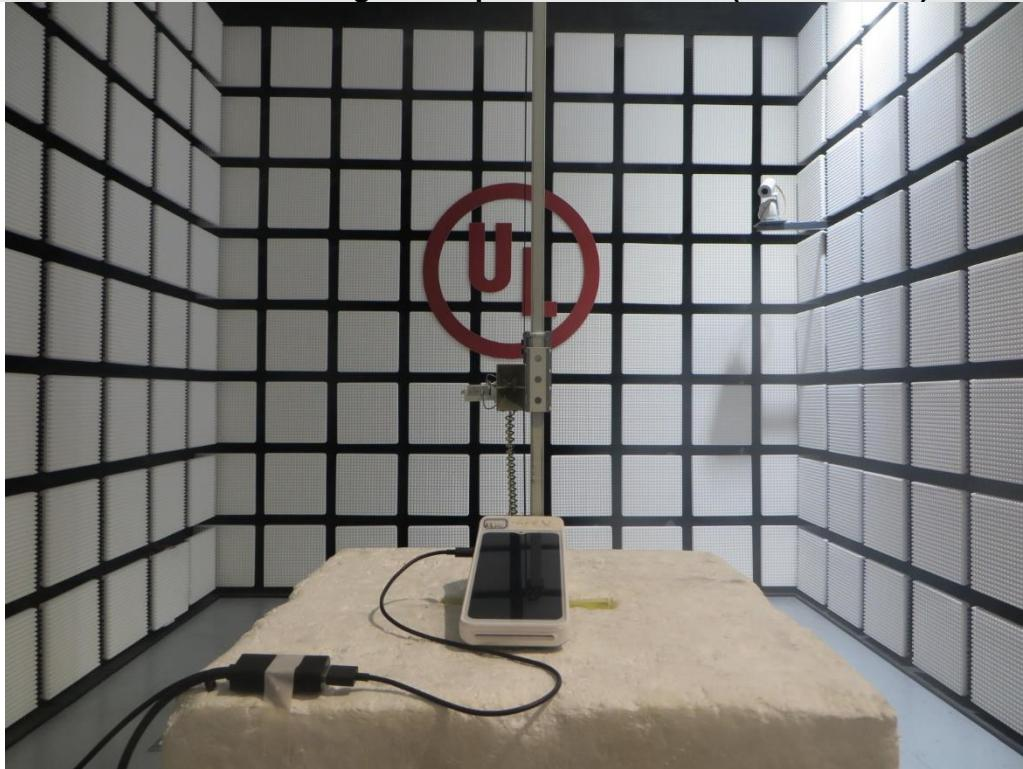
**Radiated Band edge and Spurious Emission (Above 30 MHz and Below 1 GHz)**
