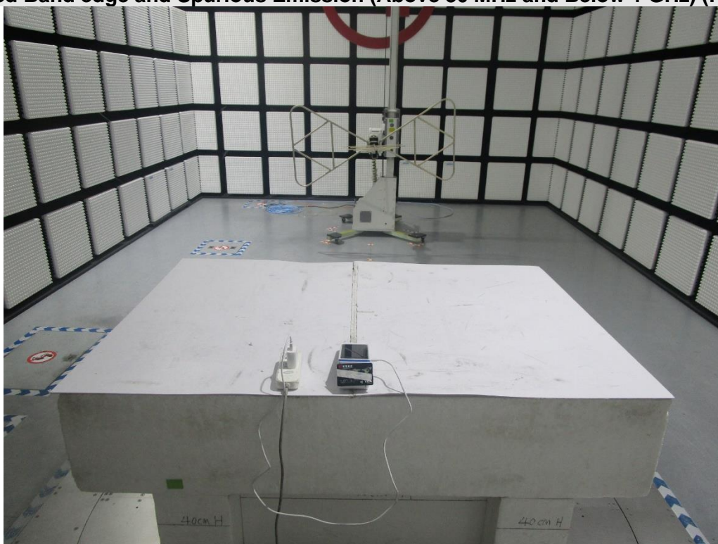
Radiated Band edge and Spurious Emission (Above 30 MHz and Below 1 GHz) (For NFC)
