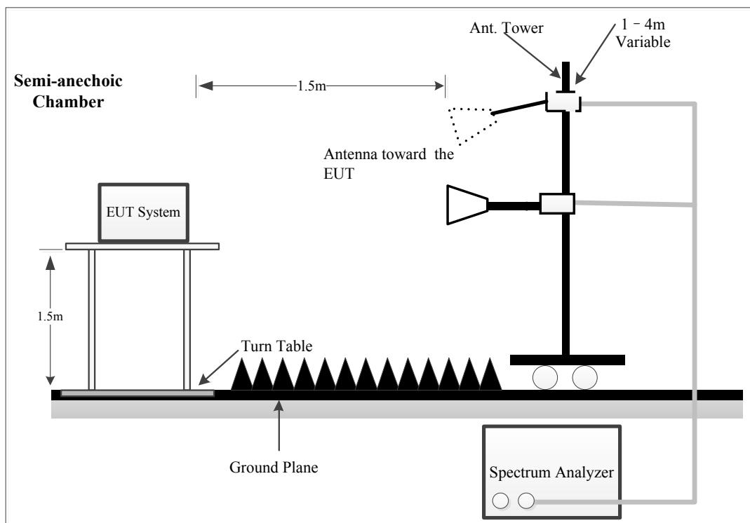
The radiated emission tests were performed in the semi-anechoic chamber, using the setup accordance with the ANSI C63.10-2013. The specification used was FCC 15.209, FCC 15.407 limits.
