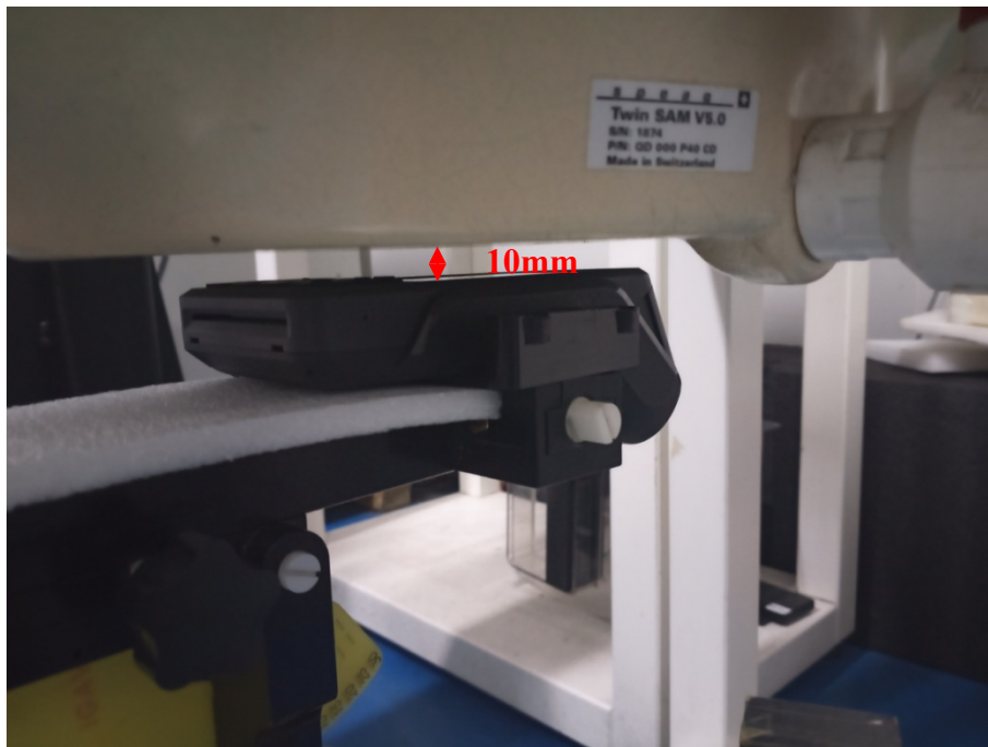
Body Front Setup Photo(10mm)
