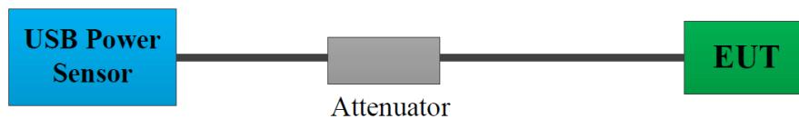
A short RF cable with low cable loss connected to the EUT antenna port, which was provided by manufacturer. The cable loss of this RF cable was offset into the setting of test equipment, which was provided by manufacturer▲.
