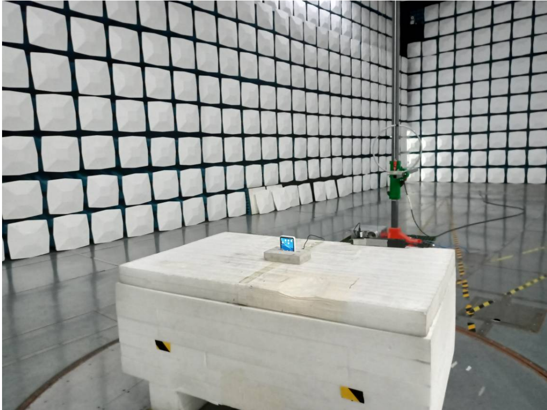
Radiated Emission 9k-30MHz Perpendicular View
