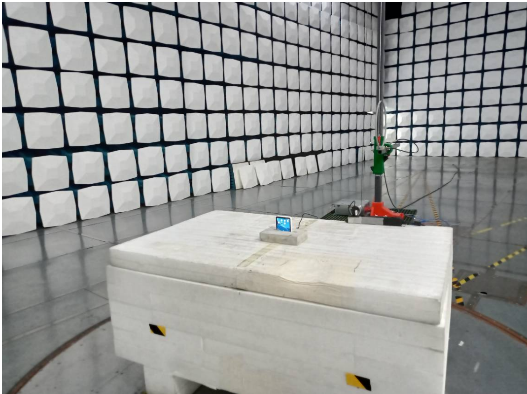
Radiated Emission 9k-30MHz Perpendicular View
