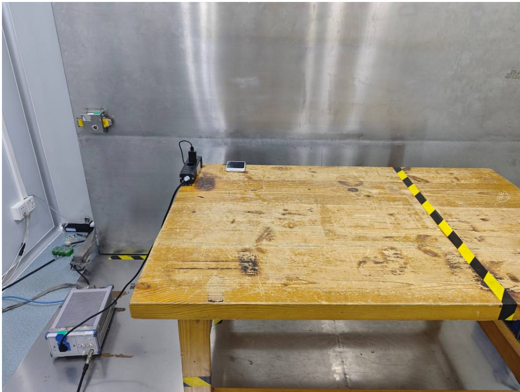
Conducted Emissions Side View
