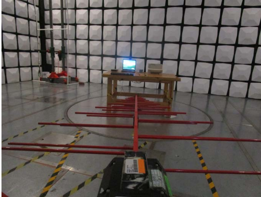
Radiated Emission Front View (Below 1GHz)
