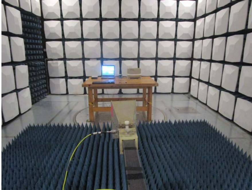
Radiated Emission Front View (Above 1GHz)
