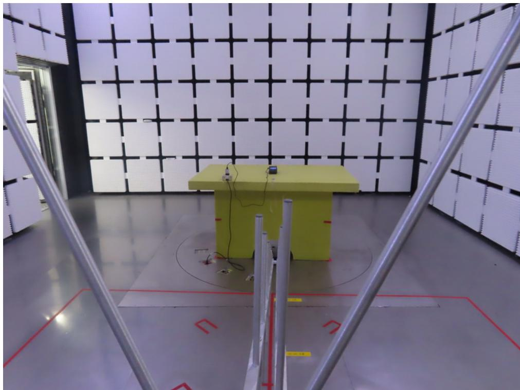
**Radiated Emissions Test Photos****1 GHz to 18 GHz**
