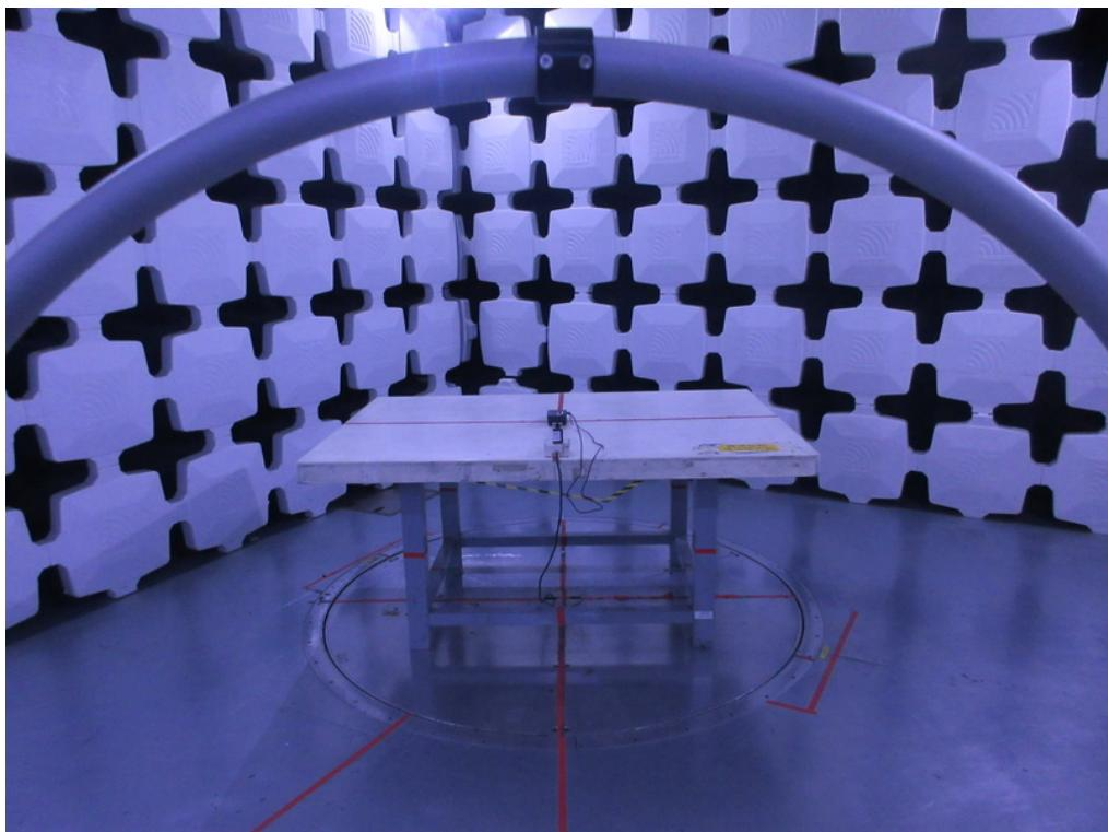
**Radiated Emissions Test Photos****30 MHz to 1000 MHz**
