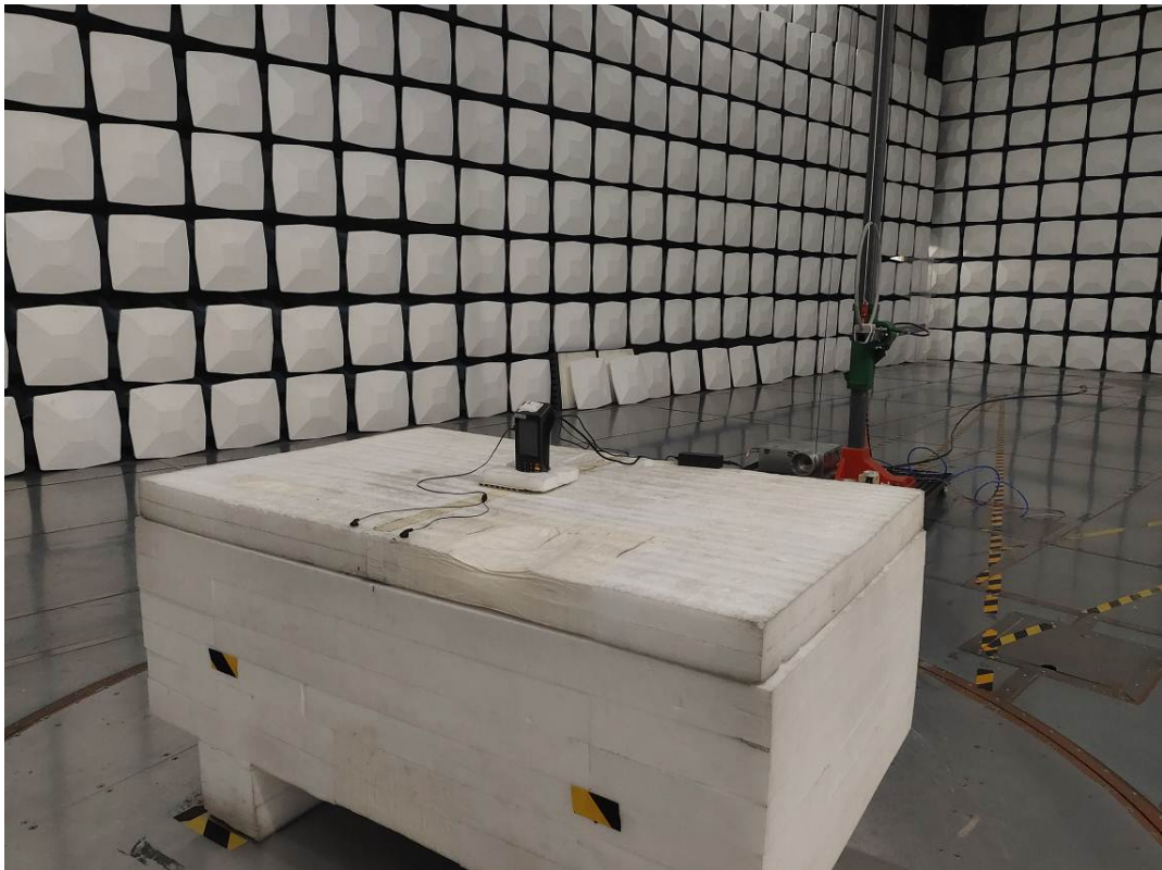
Radiated Emission 9k-30MHz Perpendicular View
