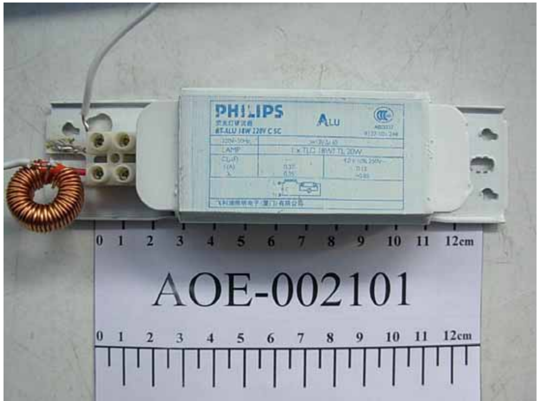
FIGURE 17 FLUORESCENT LUMINAIRES (M/N: TOP-10W) BALLAST
