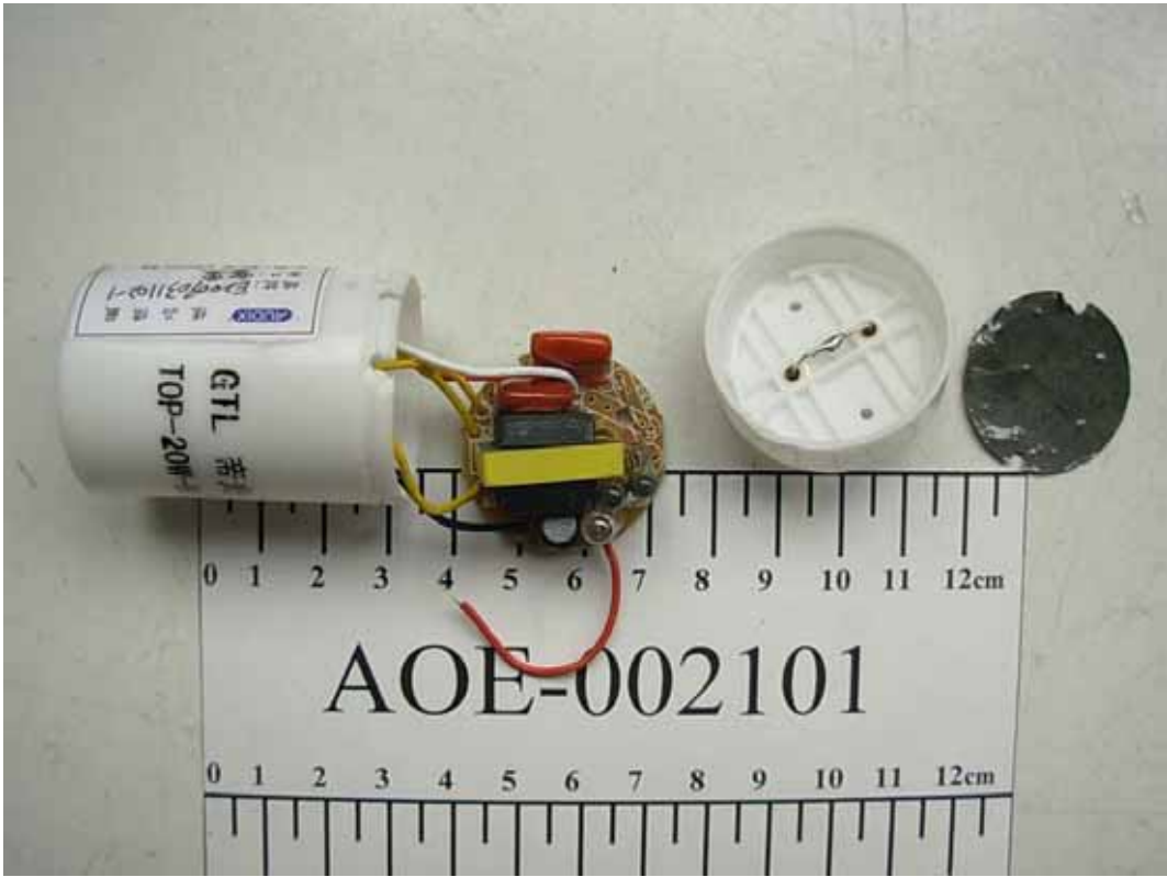
FIGURE 8 FLUORESCENT LUMINAIRES (M/N: TOP-20W) COVER REMOVED OF HEAD 1
