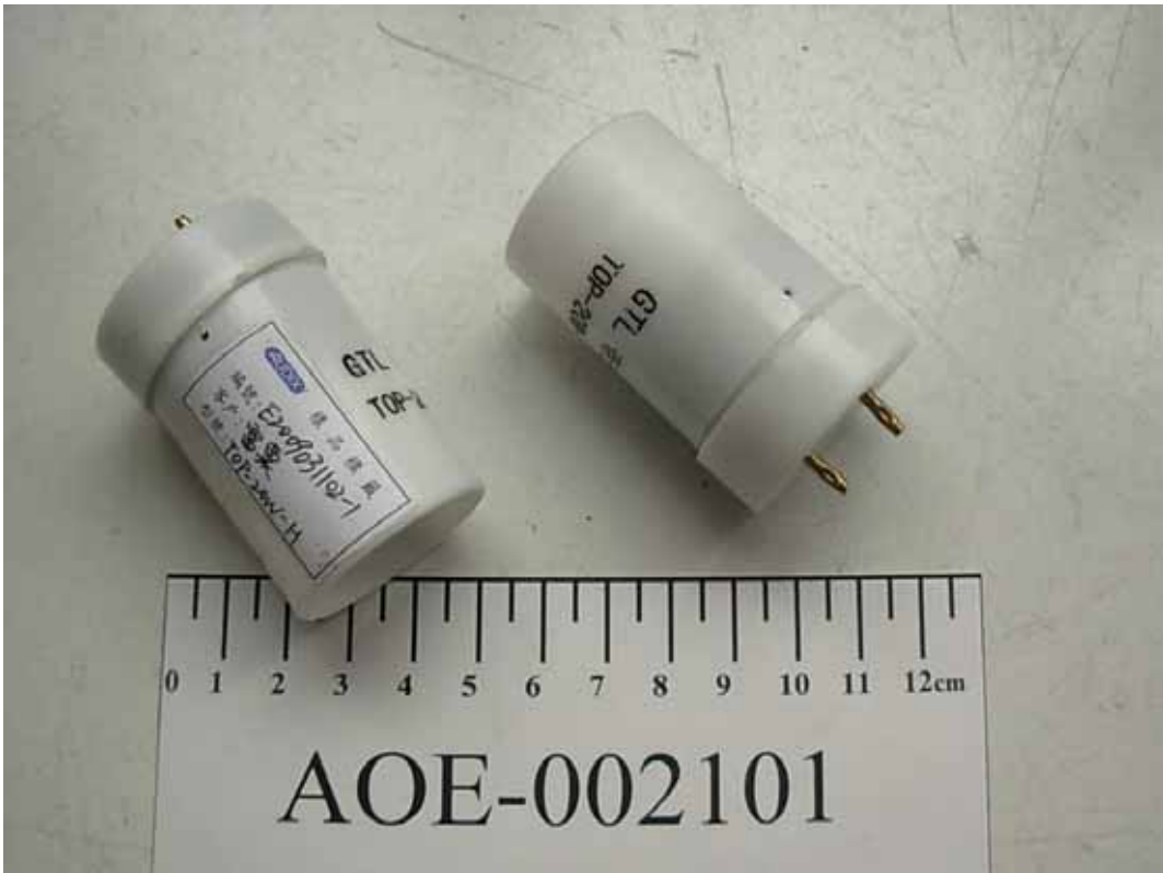
FIGURE 7 FLUORESCENT LUMINAIRES (M/N: TOP-20W) HEAD GENERAL
