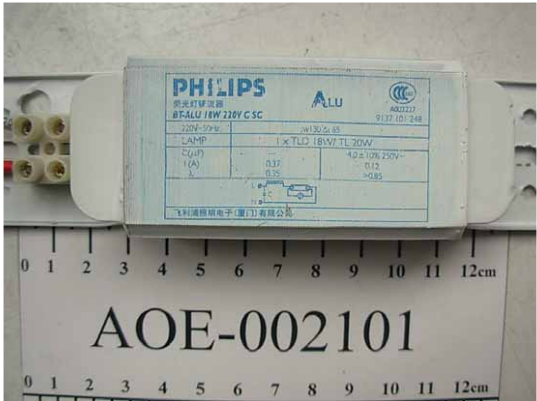
FIGURE 4 FLUORESCENT LUMINAIRES (M/N: TOP-20W) BALLAST
