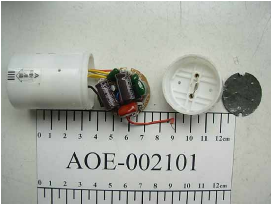
FIGURE 11 FLUORESCENT LUMINAIRES (M/N: TOP-20W) COVER REMOVE OF HEAD 2
