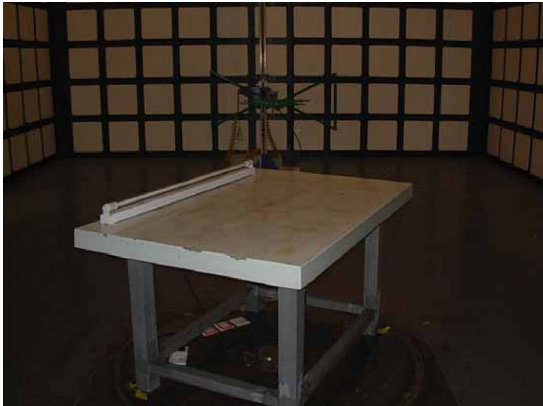
SETUP WITH MAXIMUM DETECTED EMISSION AT HORIZONTAL POLARIZATION (M/N: TOP-20W)
