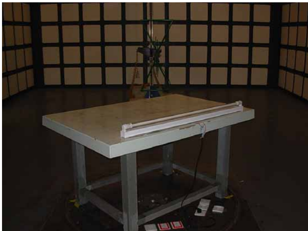
SETUP WITH MAXIMUM DETECTED EMISSION AT VERTICAL POLARIZATION (M/N: TOP-20W)
