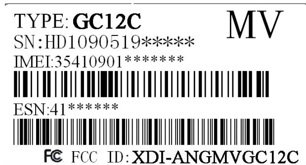
**Specifications:** Text is black or white in color and is left justified. Labels are silk-screened and shall be “permanently affixed” at a conspicuous location on the EUT.
