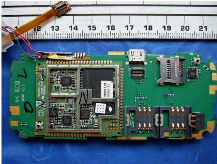
**RF Board with Shield off**
