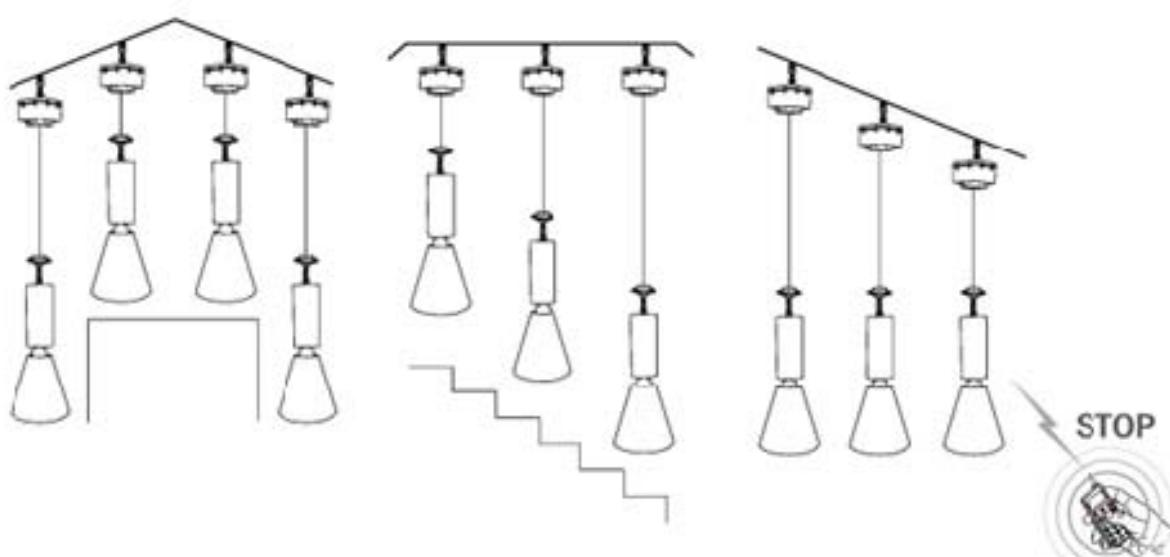
The lowering height of the lifter can be easily adjusted by pressing stop button. To set-up the lowering height, you must set the lighting fitting in the position and press down the stop button for 3 seconds till you hears the beep noise.
