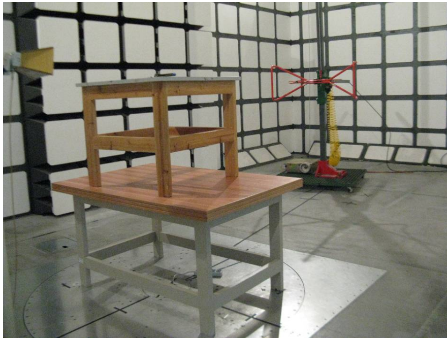
Below 1 GHz: Spurious Radiated Emissions - Rear View
