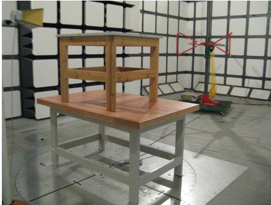
Below 1 GHz: Spurious Radiated Emissions - Rear View
