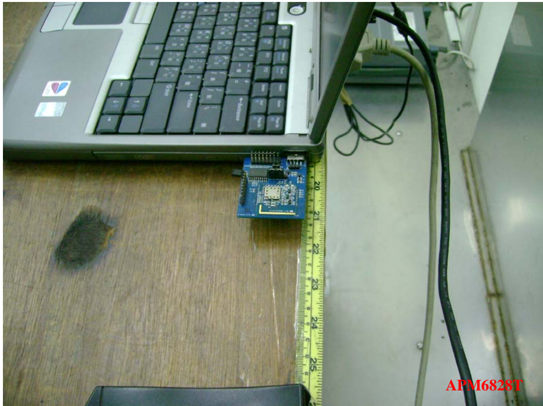
Photo 4: Conducted Emission Test Set-up photo
