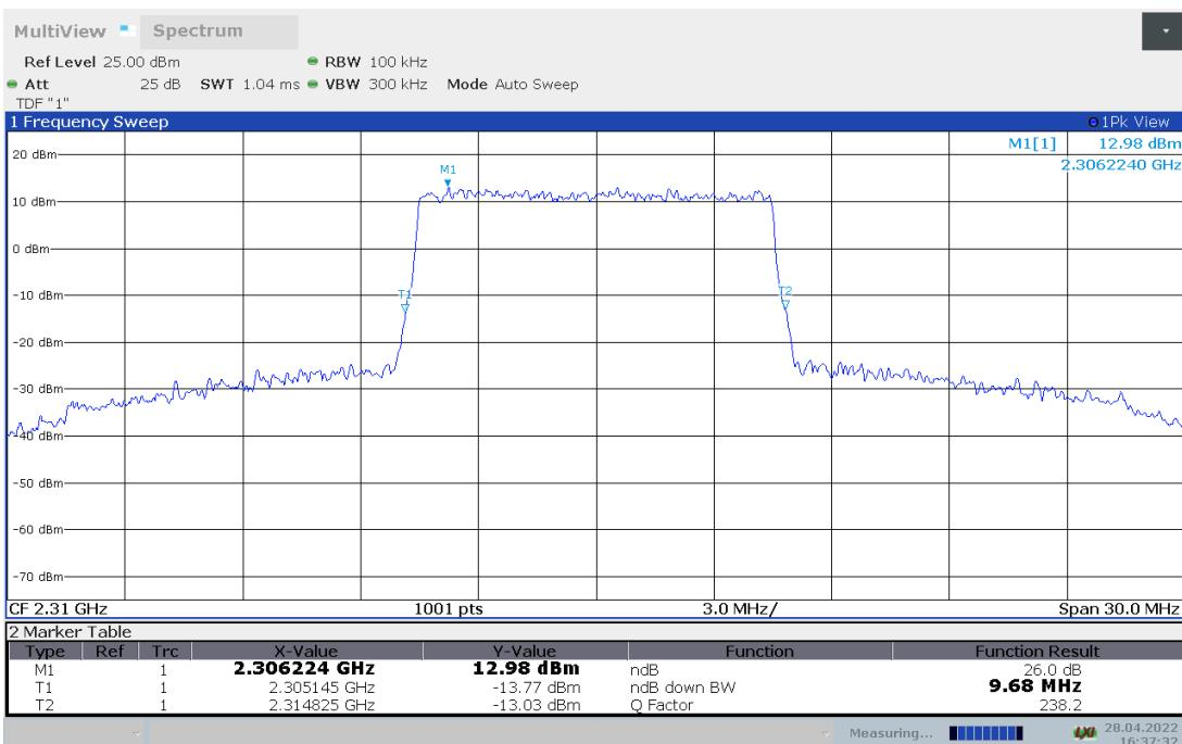
**LTE band 30, 10MHz Bandwidth, 64QAM (-26dBc BW)**
