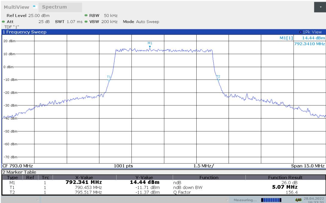
**LTE band 14, 5MHz Bandwidth,64QAM (-26dBc BW)**
