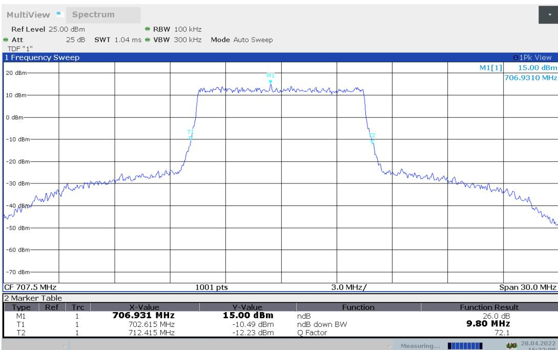
**LTE band 12, 10MHz Bandwidth, 64QAM (-26dBc BW)**
