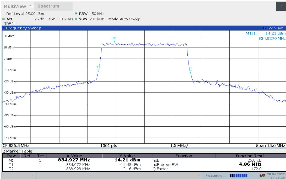
**LTE band 5, 5MHz Bandwidth,64QAM (-26dBc BW)**
