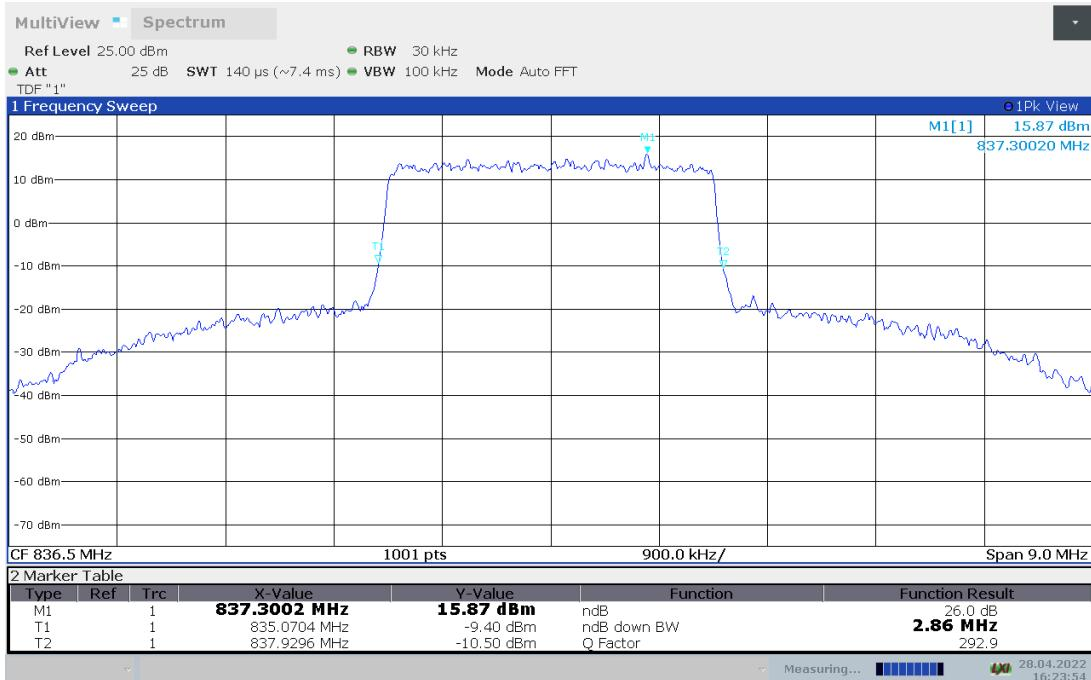
**LTE band 5, 3MHz Bandwidth, 16QAM (-26dBc BW)**
