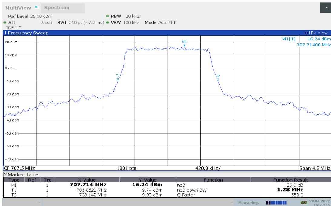
**LTE band 12, 1.4MHz Bandwidth, 16QAM (-26dBc BW)**
