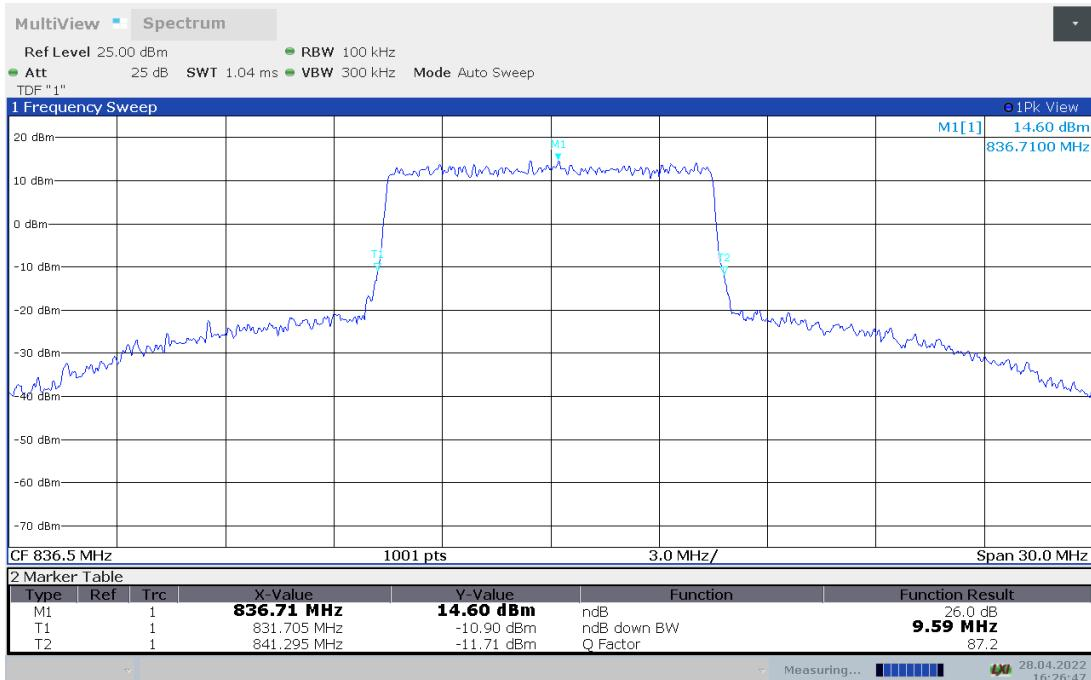
**LTE band 5, 10MHz Bandwidth, 64QAM (-26dBc BW)**
