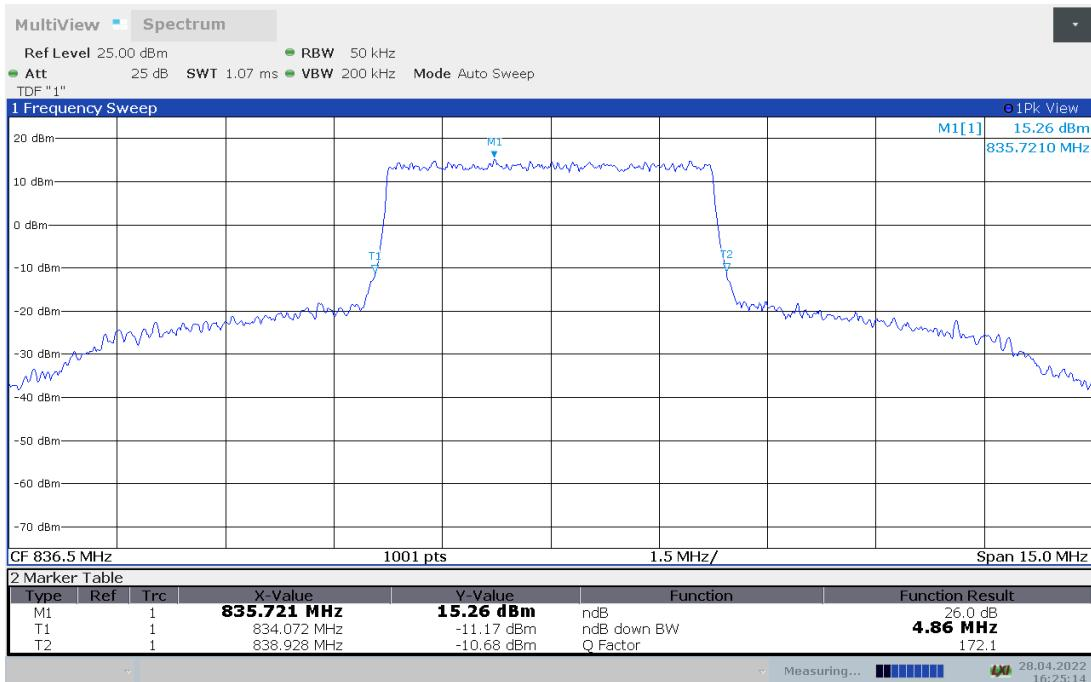
**LTE band 5, 5MHz Bandwidth,16QAM (-26dBc BW)**
