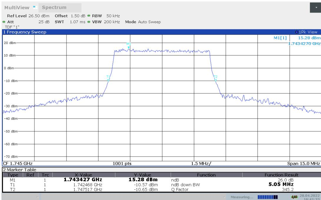
**LTE band 66, 5MHz Bandwidth,64QAM (-26dBc BW)**
