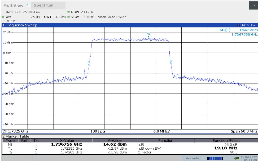
**LTE band 4, 20MHz Bandwidth, 16QAM (-26dBc BW)**
