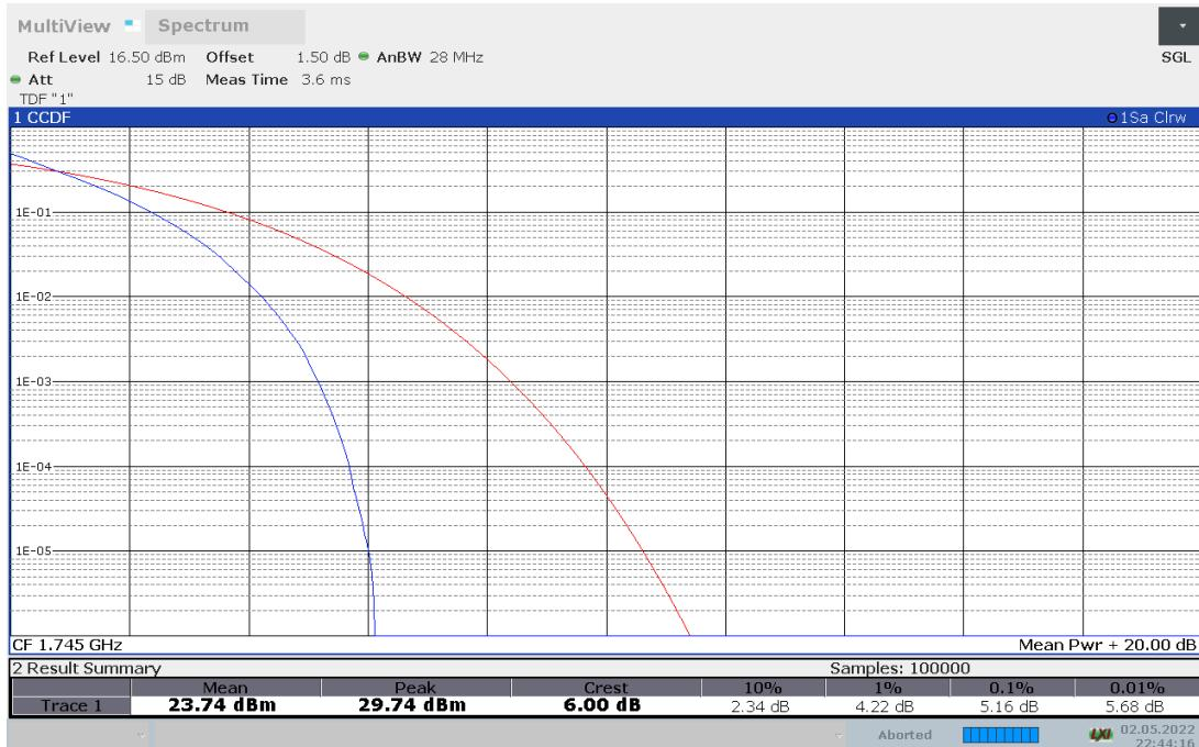
**LTE band 66, 20MHz Bandwidth, 16QAM (PAPR)**
