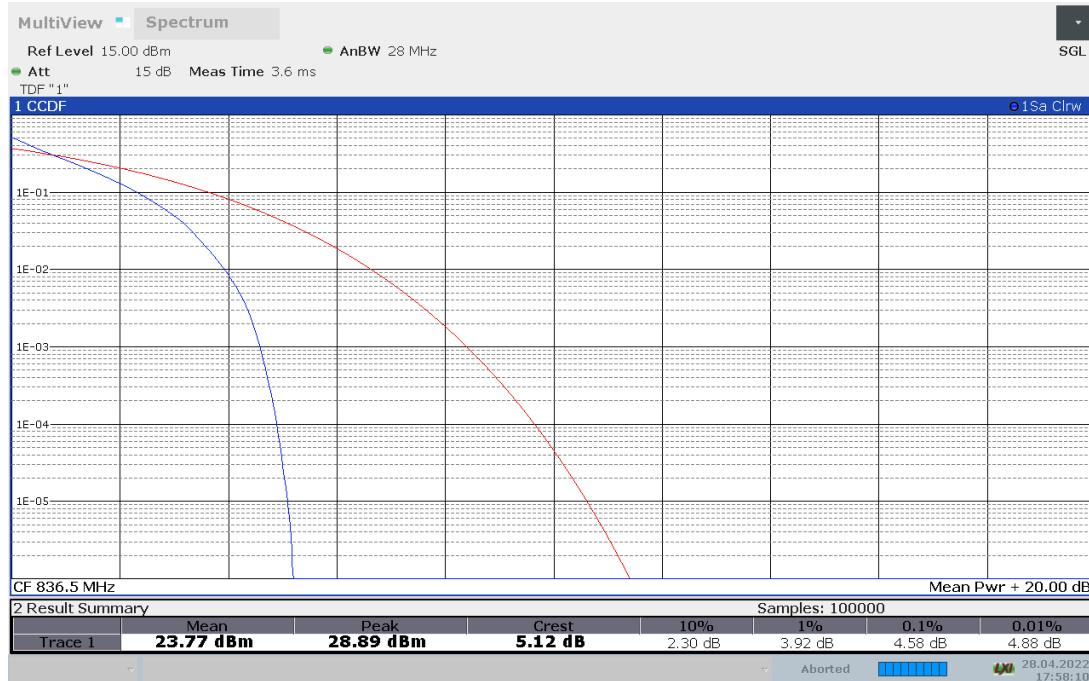
**LTE band 5, 10MHz Bandwidth, 16QAM (PAPR)**
