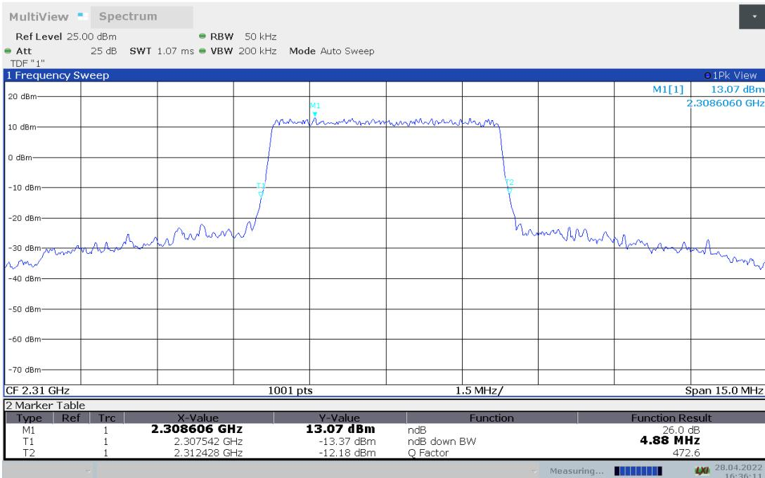
**LTE band 30, 5MHz Bandwidth,64QAM (-26dBc BW)**
