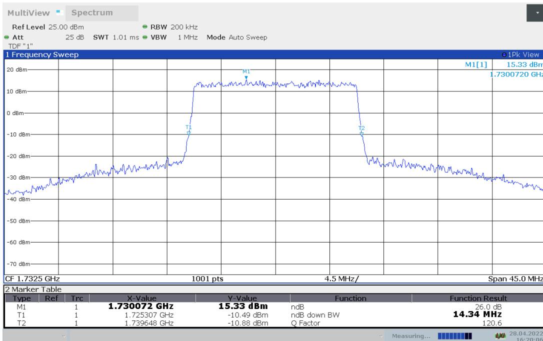
**LTE band 4, 15MHz Bandwidth, 64QAM (-26dBc BW)**
