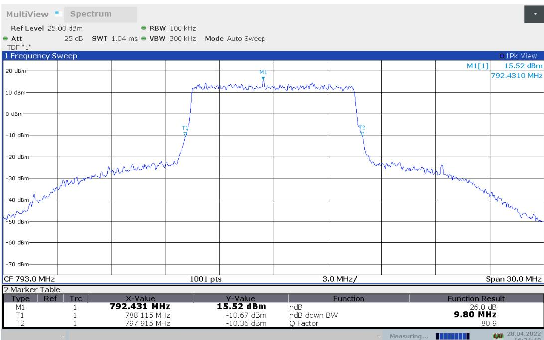
**LTE band 14, 10MHz Bandwidth, 64QAM (-26dBc BW)**
