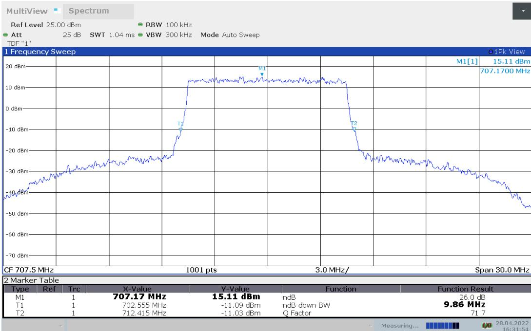
**LTE band 12, 10MHz Bandwidth, 16QAM (-26dBc BW)**
