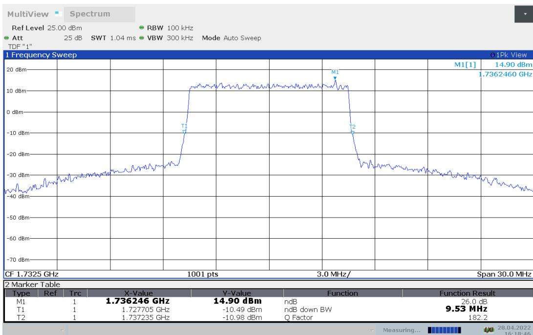
**LTE band 4, 10MHz Bandwidth, 64QAM (-26dBc BW)**
