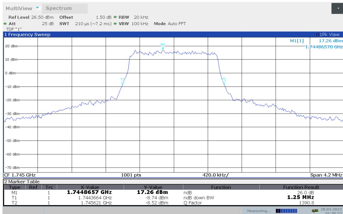
**LTE band 66, 1.4MHz Bandwidth, 64QAM (-26dBc BW)**
