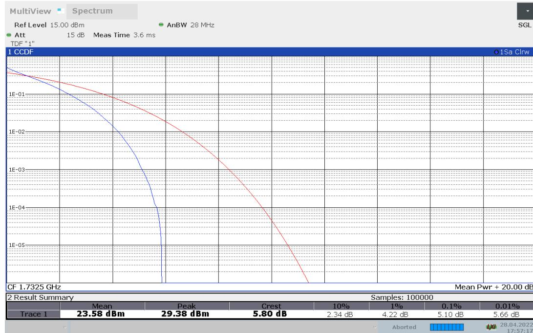
**LTE band 4, 20MHz Bandwidth, 16QAM (PAPR)**
