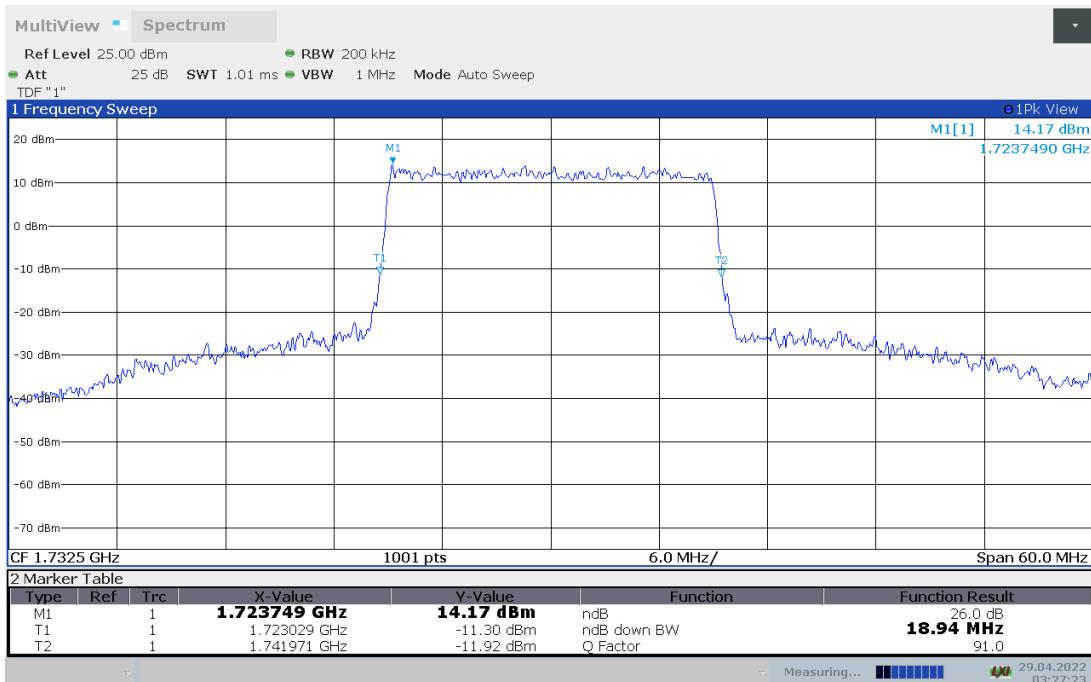
**LTE band 4, 20MHz Bandwidth, 64QAM (-26dBc BW)**
