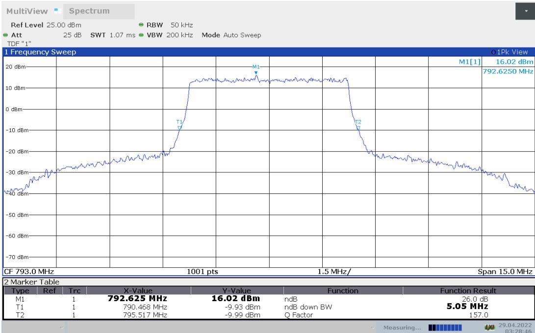
**LTE band 14, 5MHz Bandwidth,16QAM (-26dBc BW)**
