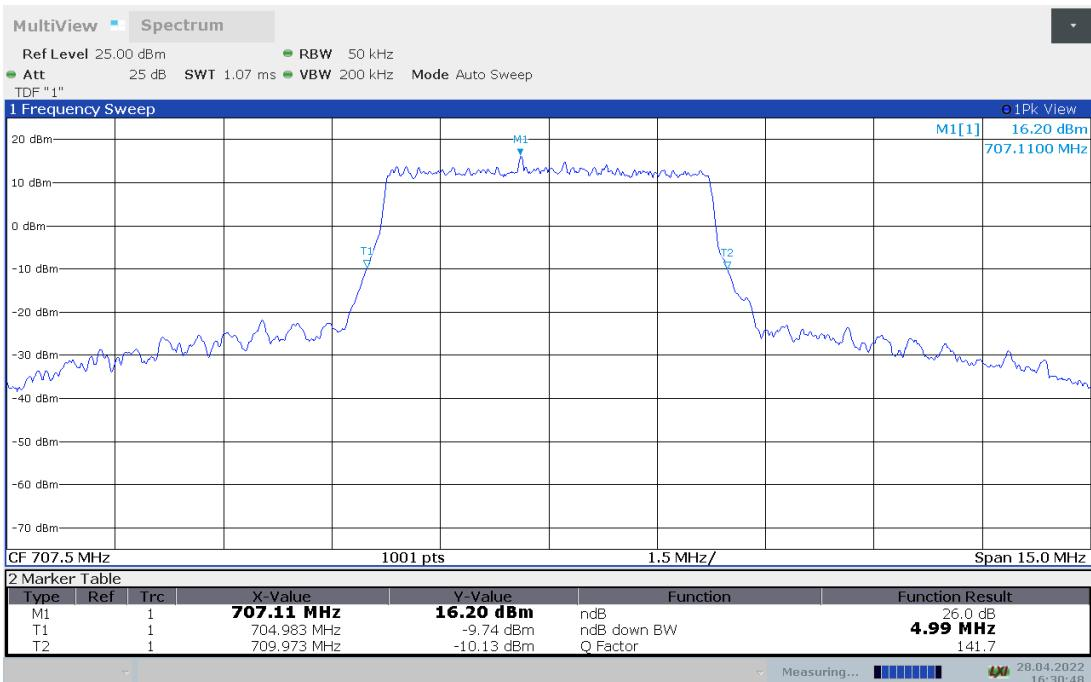
**LTE band 12, 5MHz Bandwidth,64QAM (-26dBc BW)**
