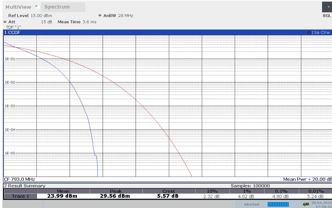
**LTE band 14, 10MHz Bandwidth, 16QAM (PAPR)**
