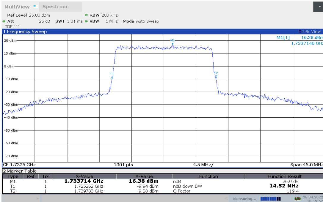
**LTE band 4, 15MHz Bandwidth, 16QAM (-26dBc BW)**
