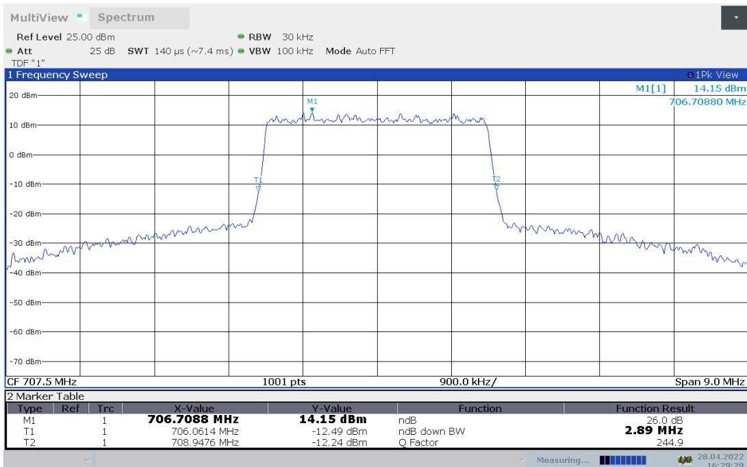
**LTE band 12, 3MHz Bandwidth, 64QAM (-26dBc BW)**
