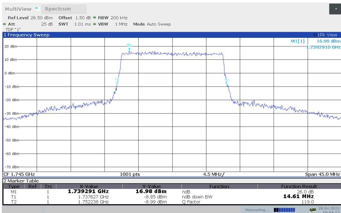
**LTE band 66, 15MHz Bandwidth, 64QAM (-26dBc BW)**
