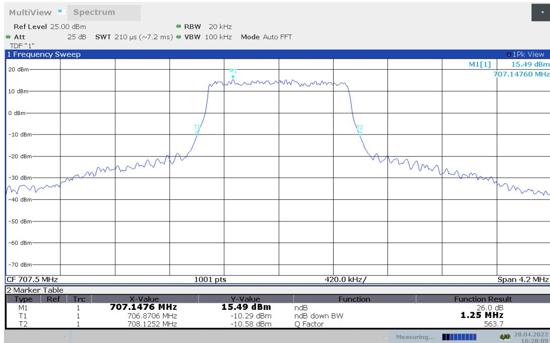
**LTE band 12, 1.4MHz Bandwidth, 64QAM (-26dBc BW)**
