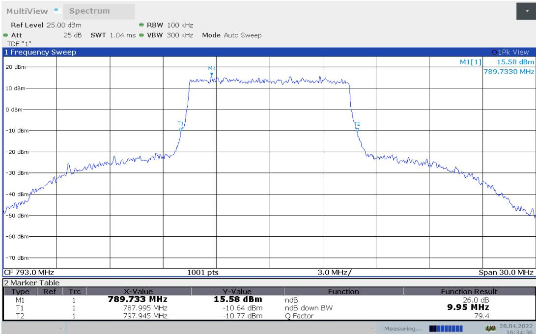
**LTE band 14, 10MHz Bandwidth, 16QAM (-26dBc BW)**
