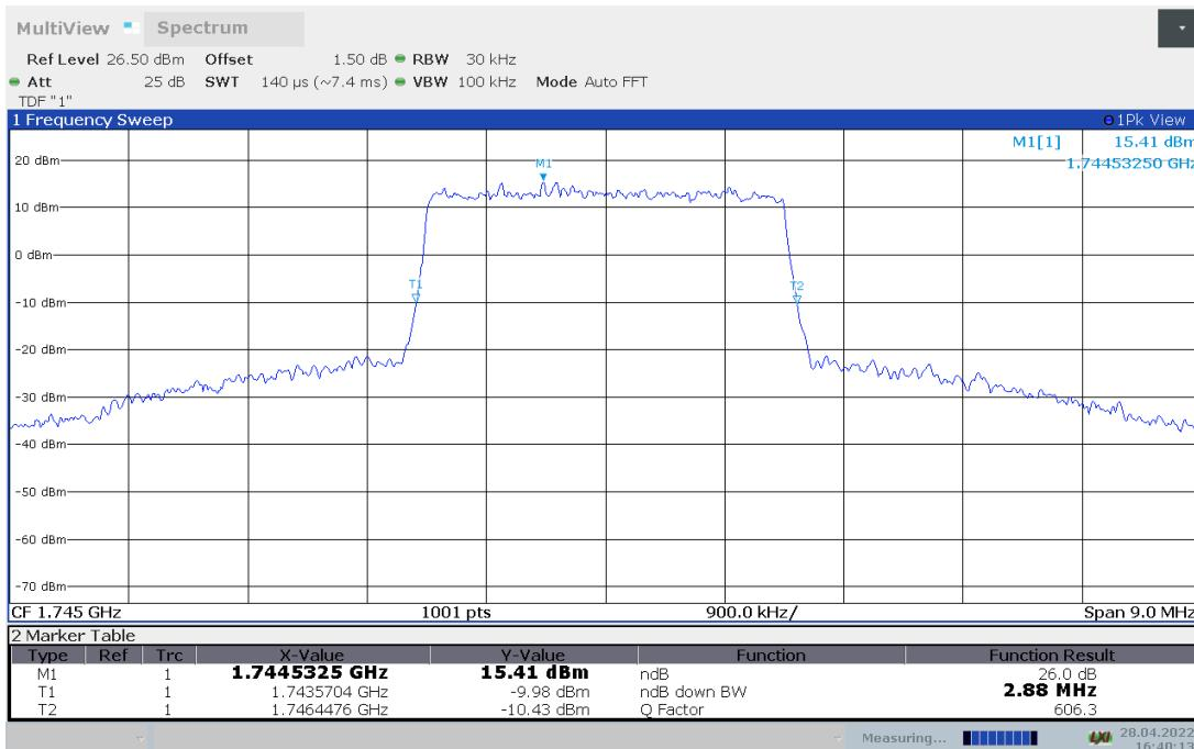
**LTE band 66, 3MHz Bandwidth, 64QAM (-26dBc BW)**
