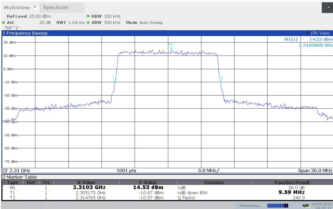
**LTE band 30, 10MHz Bandwidth, 16QAM (-26dBc BW)**
