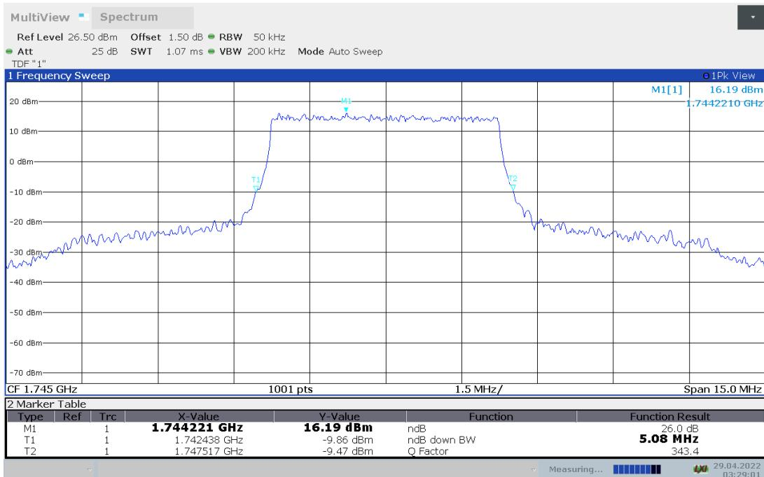
**LTE band 66, 5MHz Bandwidth,16QAM (-26dBc BW)**
