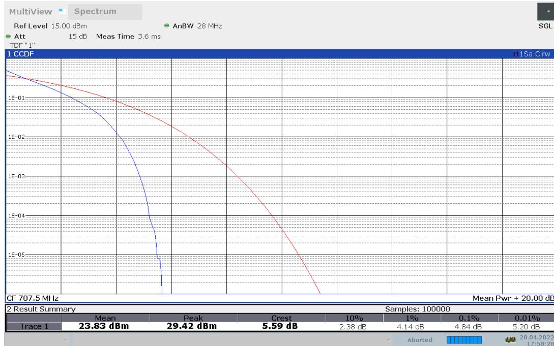
**LTE band 12, 10MHz Bandwidth, 16QAM (PAPR)**
