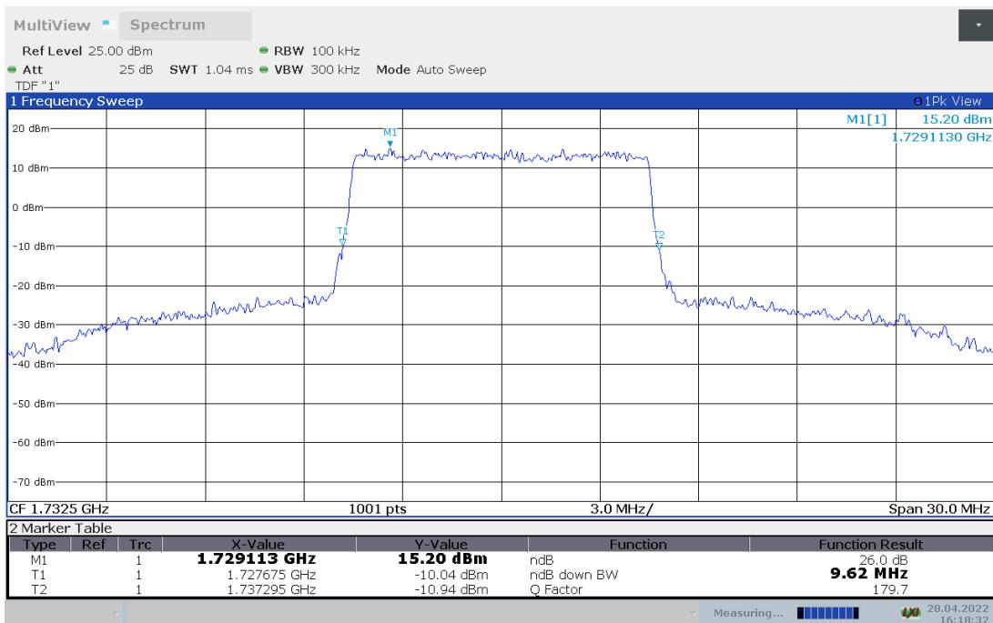
**LTE band 4, 10MHz Bandwidth, 16QAM (-26dBc BW)**
