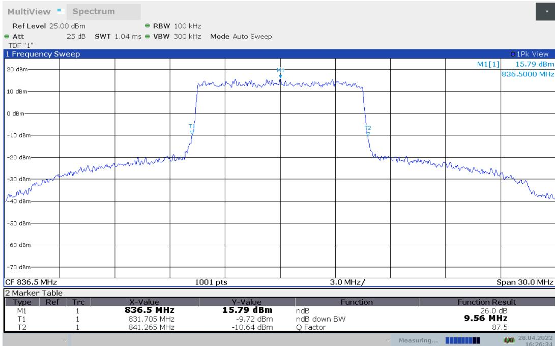
**LTE band 5, 10MHz Bandwidth, 16QAM (-26dBc BW)**
