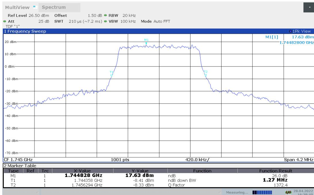
**LTE band 66, 1.4MHz Bandwidth, 16QAM (-26dBc BW)**
