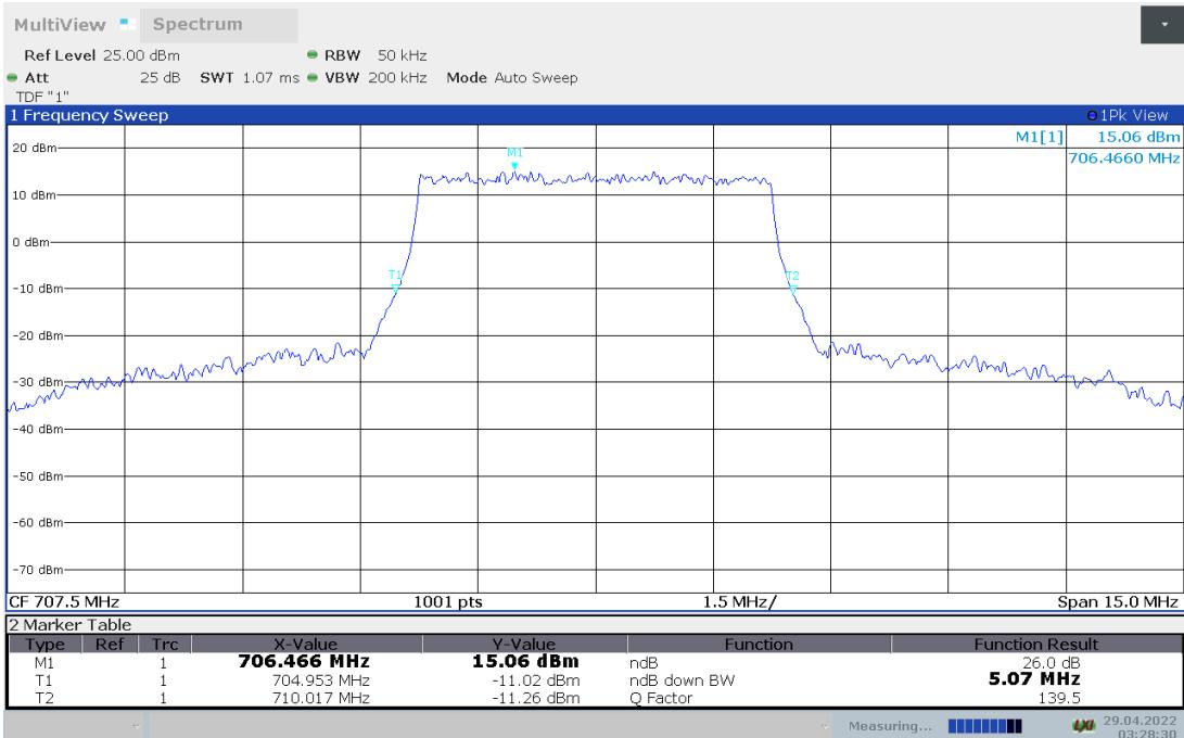
**LTE band 12, 5MHz Bandwidth,16QAM (-26dBc BW)**
