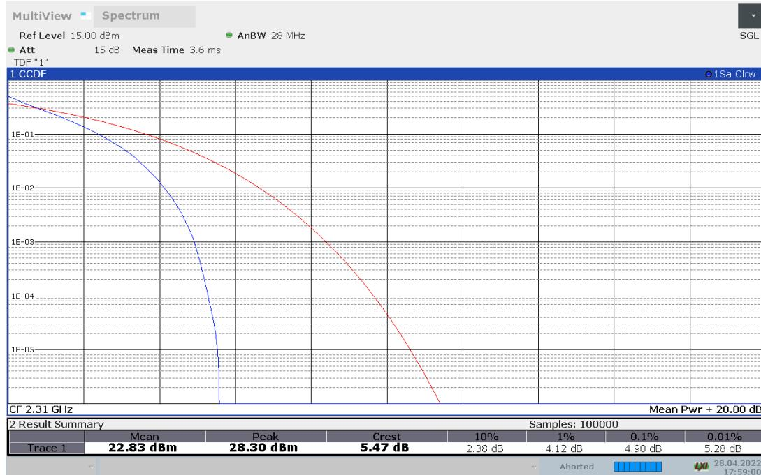
**LTE band 30, 10MHz Bandwidth, 16QAM (PAPR)**
