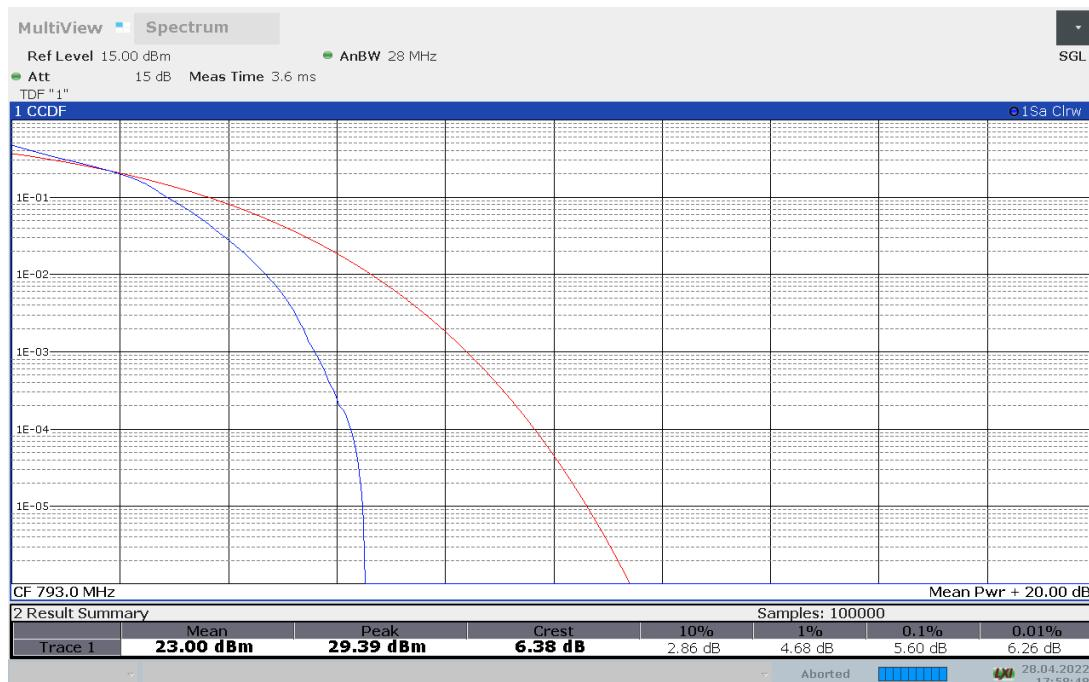
**LTE band 14, 10MHz Bandwidth, 64QAM (PAPR)**
