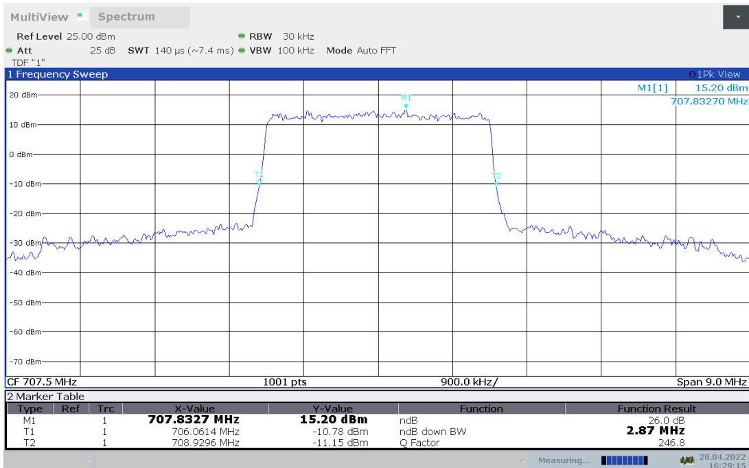
**LTE band 12, 3MHz Bandwidth, 16QAM (-26dBc BW)**
