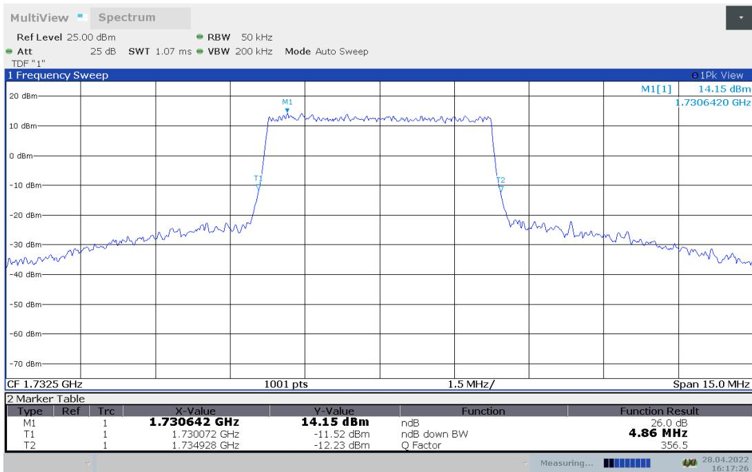
**LTE band 4, 5MHz Bandwidth,64QAM (-26dBc BW)**
