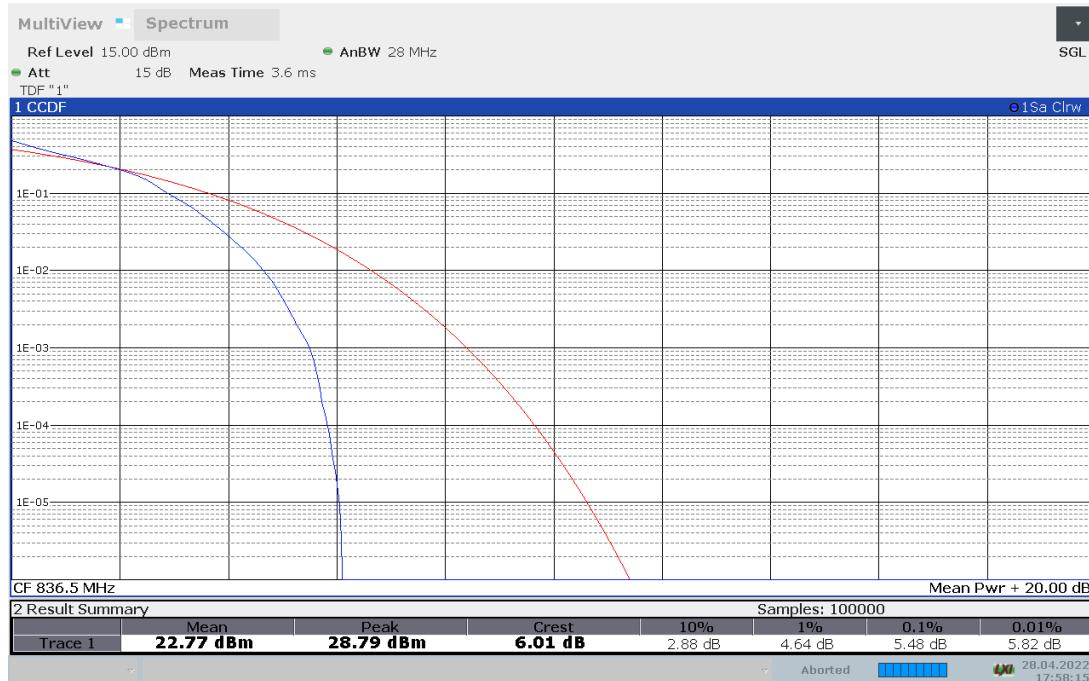
**LTE band 5, 10MHz Bandwidth, 64QAM (PAPR)**
