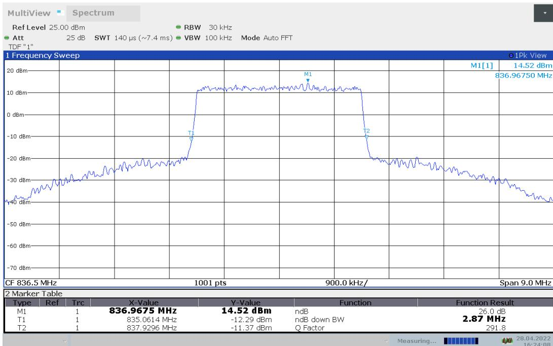
**LTE band 5, 3MHz Bandwidth, 64QAM (-26dBc BW)**
