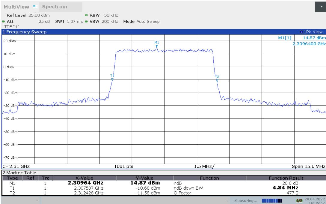
**LTE band 30, 5MHz Bandwidth,16QAM (-26dBc BW)**
