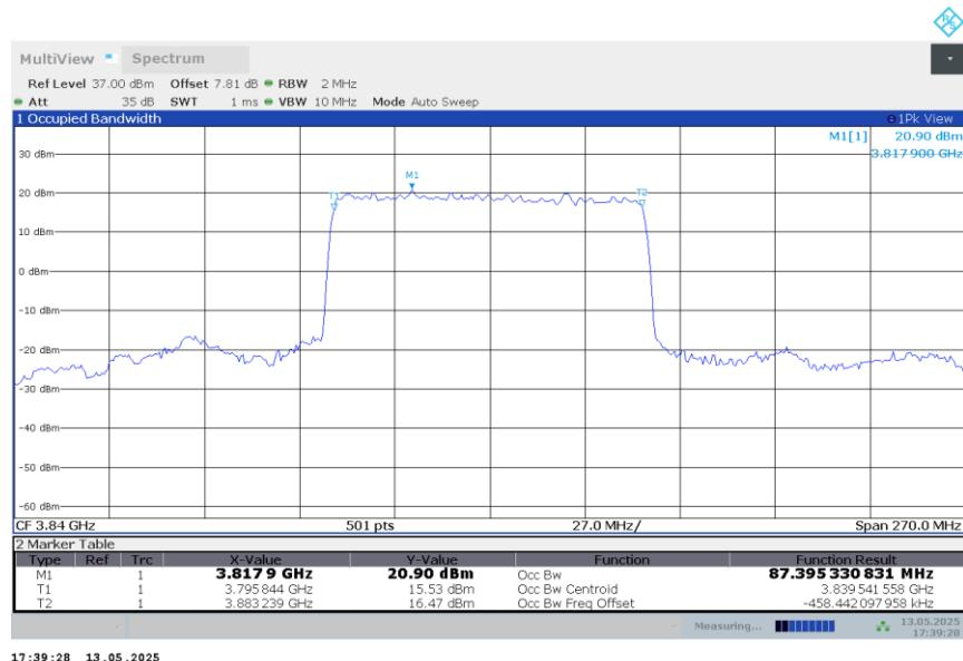
**n77H,90MHz Bandwidth,DFT-s-QPSK (99% BW)**
