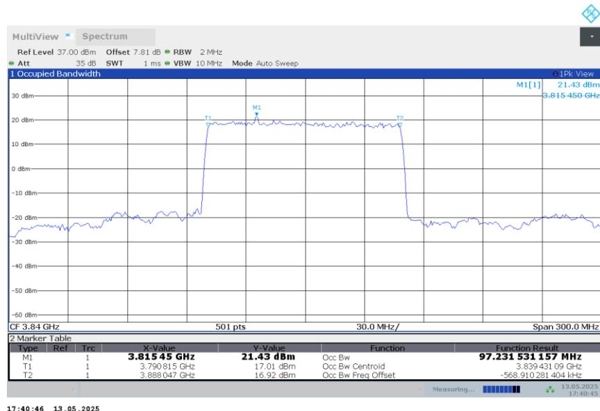
**n77H,100MHz Bandwidth,DFT-s-QPSK (99% BW)**
