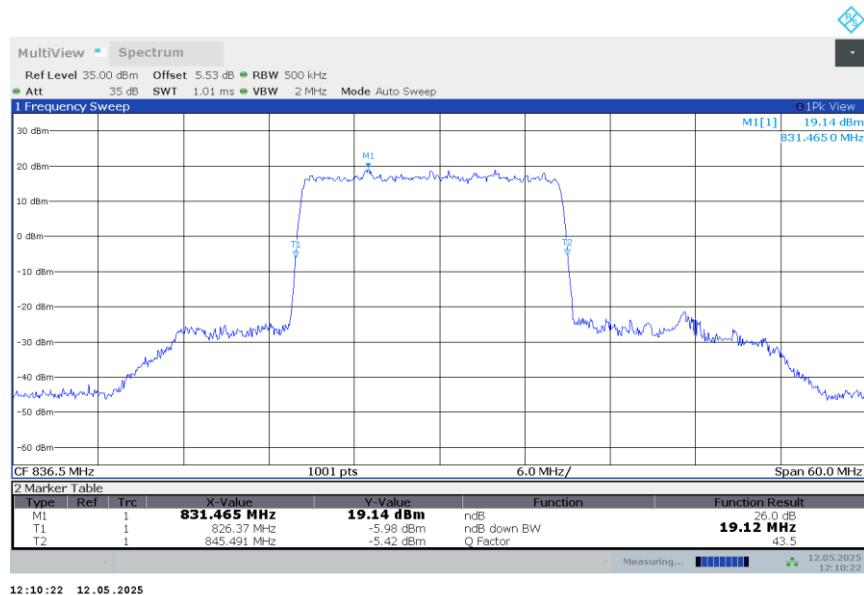
n5,20MHz Bandwidth,DFT-s-QPSK (-26dBc BW)
