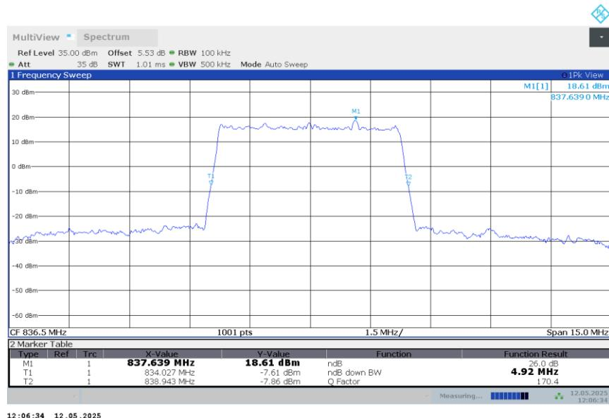
n5,5MHz Bandwidth,DFT-s-QPSK (-26dBc BW)
