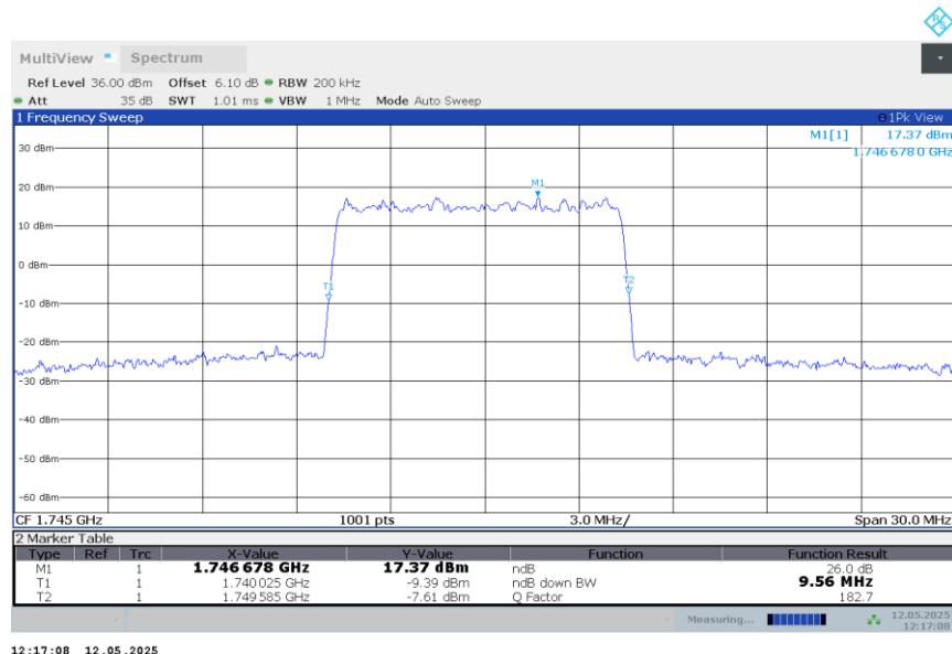
**n66,10MHz Bandwidth,DFT-s-16QAM (-26dBc BW)**
