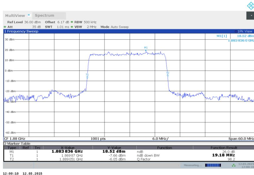
**n2,20MHz Bandwidth,DFT-s-QPSK (-26dBc BW)**
