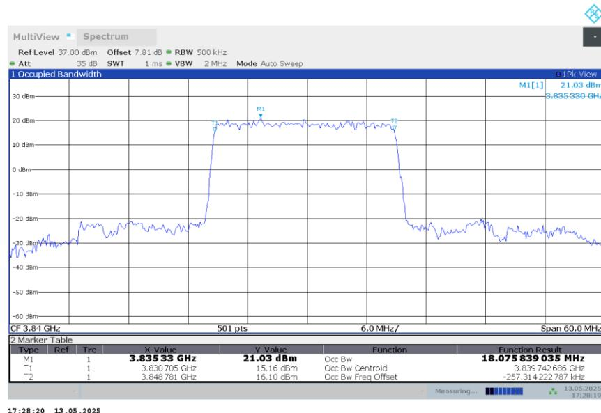
**n77H,20MHz Bandwidth,DFT-s-QPSK (99% BW)**
