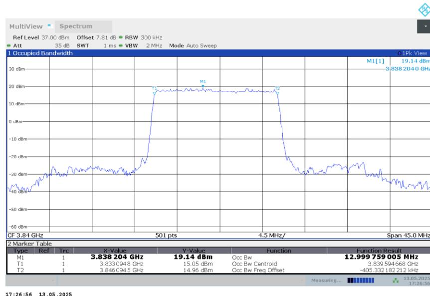
**n77H,15MHz Bandwidth,DFT-s-QPSK (99% BW)**
