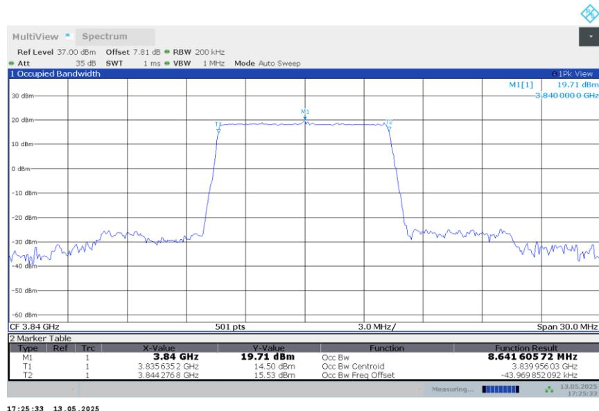
**n77H,10MHz Bandwidth,DFT-s-QPSK (99% BW)**
