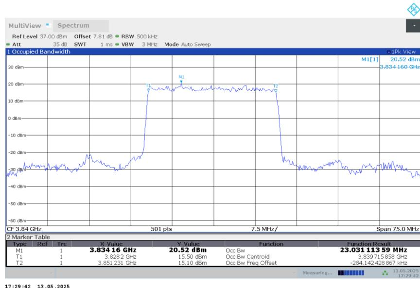
**n77H,25MHz Bandwidth,DFT-s-QPSK (99% BW)**
