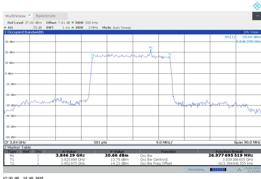
**n77H,30MHz Bandwidth,DFT-s-QPSK (99% BW)**
