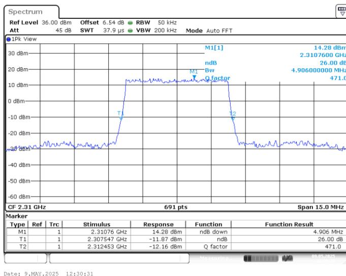
**LTE band 30 , 5MHz Bandwidth,MID,16QAM (-26dBc BW)**
