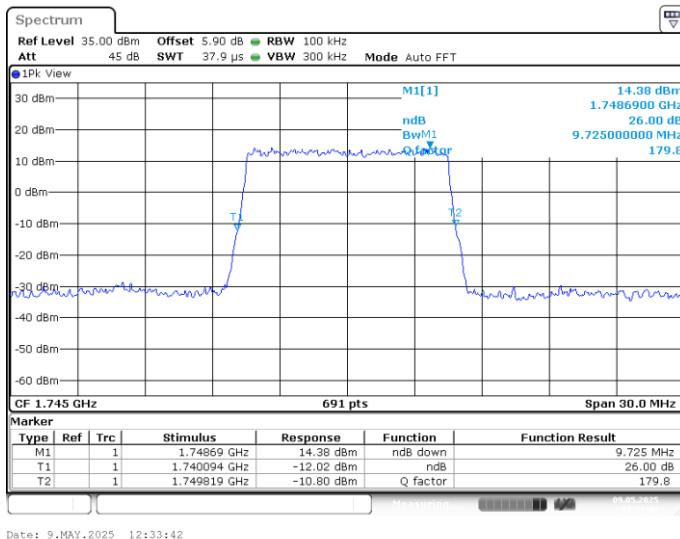
**LTE band 66 , 10MHz Bandwidth,MID,16QAM (-26dBc BW)**
