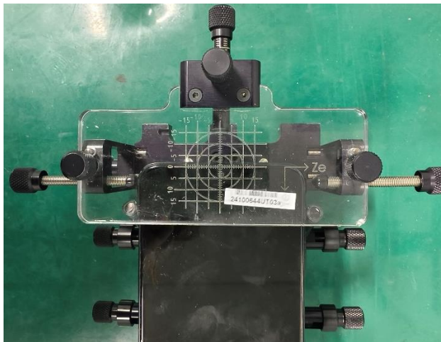
Pic 3: Handset Positioner (HHPIII) with mounted EUT mobile phone
