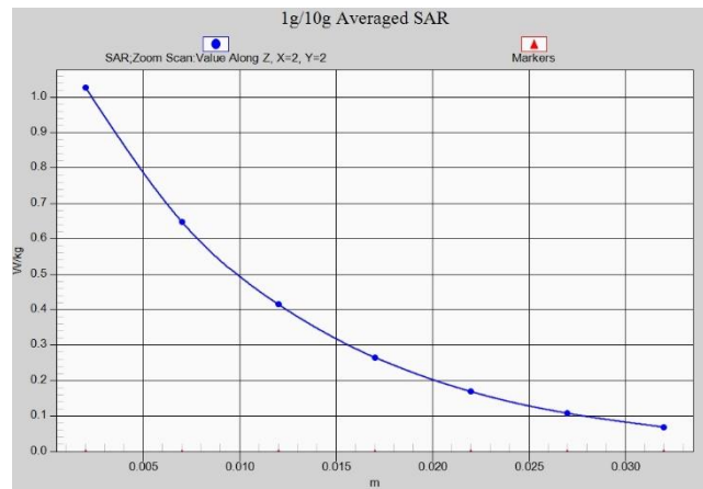
Fig.A.1- 10 Z-Scan at power reference point (W1700) 15mm
