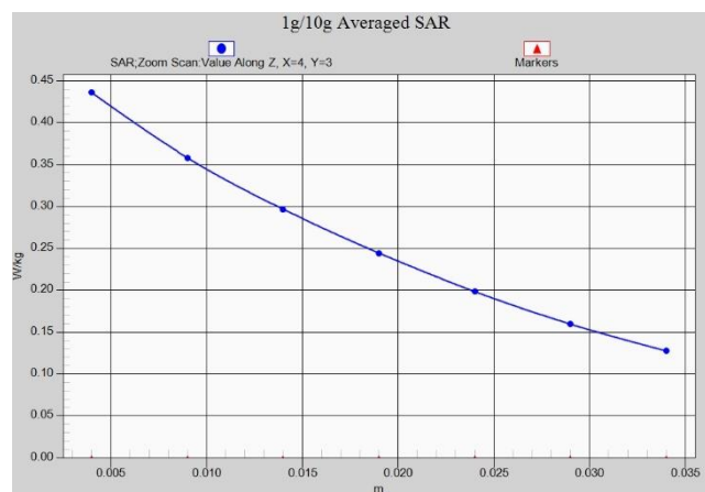
Fig.A.1- 12 Z-Scan at power reference point (W850)
