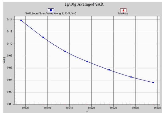
Fig.A.1- 1 Z-Scan at power reference point (GSM850)
