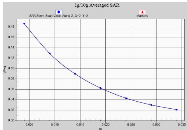
Fig.A.1- 17 Z-Scan at power reference point (LTE band4)
