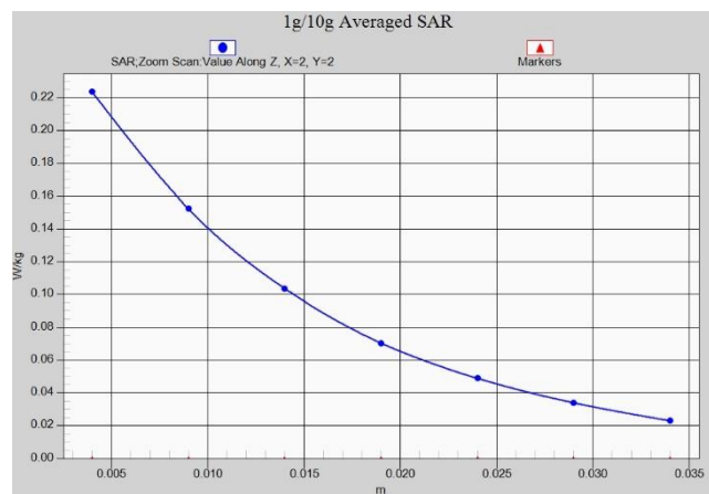
Fig.A.1- 14 Z-Scan at power reference point (LTE band2)
