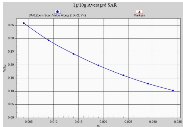
Fig.A.1- 20 Z-Scan at power reference point (LTE band5)
