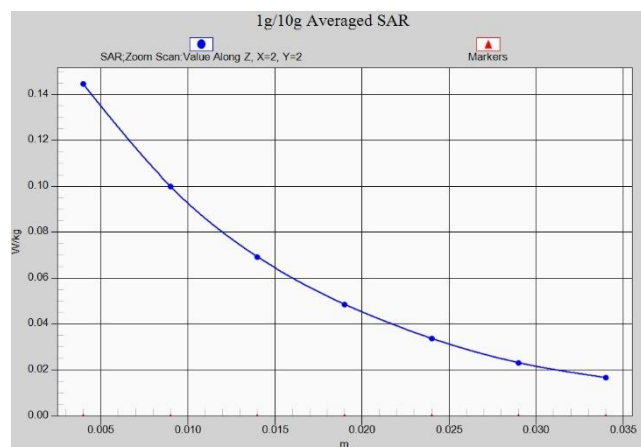
Fig.A.1- 9 Z-Scan at power reference point (W1700)
