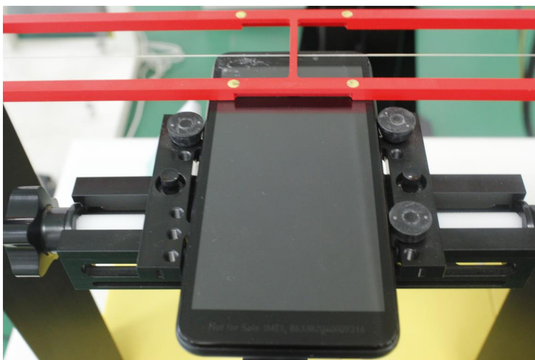
Picture 2: EUT Positioning for RF/T-coil
