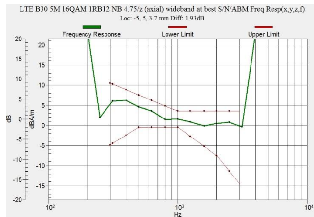
Figure C.11 Frequency Response of LTE B30
