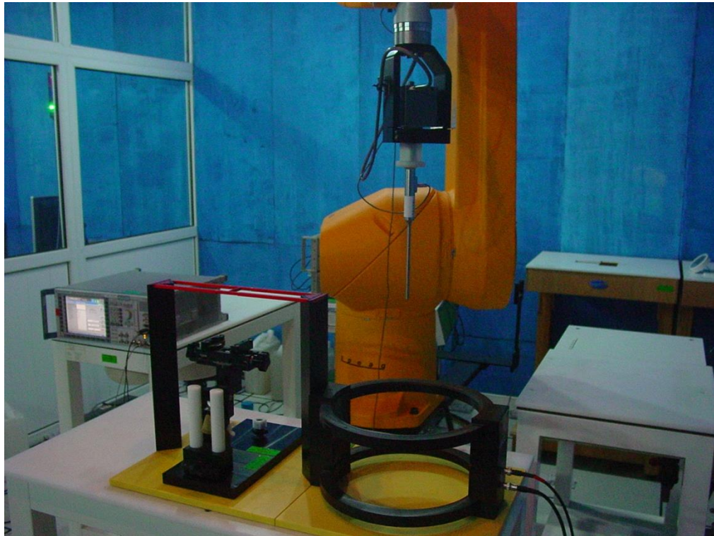
Picture A1: HAC T-Coil System Layout
