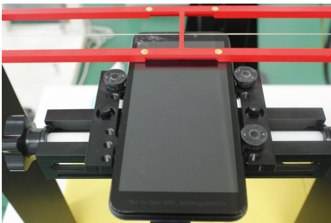
Picture 2: EUT Positioning for RF/T-coil
