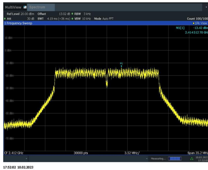
Fig.A.3.7 Power Spectral Density (802.11n-HT20, Ch 1)
