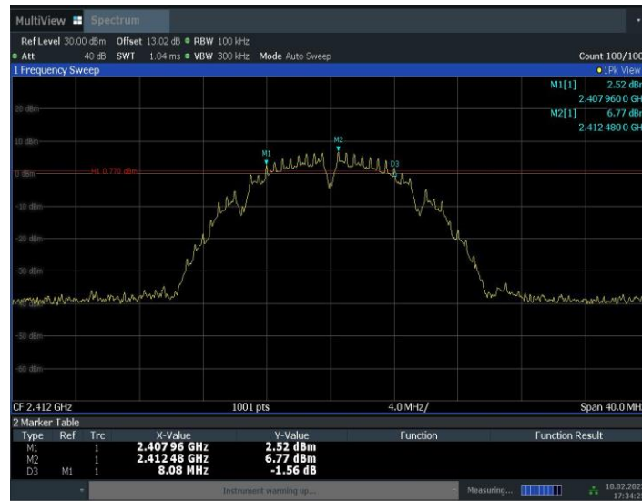
Fig.A.4.1 Occupied 6dB Bandwidth(802.11b,Ch 1)
