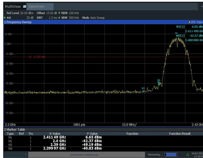
Fig.A.5.1 Band Edges (802.11b, Ch 1)
