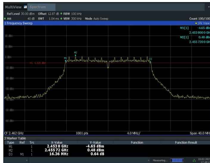
Fig.A.4.6 Occupied 6dB Bandwidth (802.11g, Ch 11)
