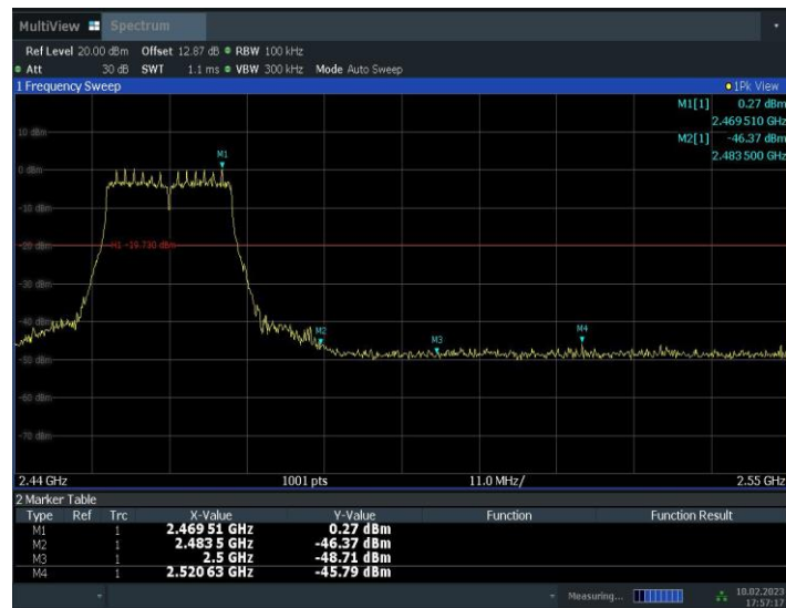
Fig.A.5.6 Band Edges (802.11n-HT20, Ch 11)
