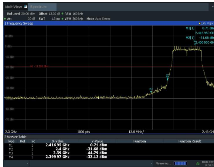
Fig.A.5.5 Band Edges (802.11n-HT20, Ch 1)
