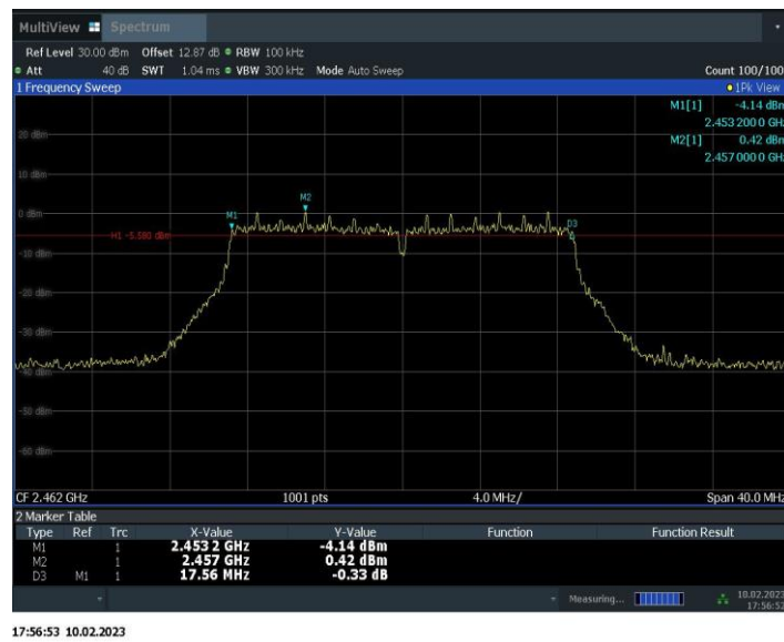
Fig.A.4.9 Occupied 6dB Bandwidth (802.11n-HT20, Ch 11)
