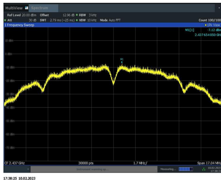
Fig.A.3.2 Power Spectral Density (802.11b, Ch 6)
