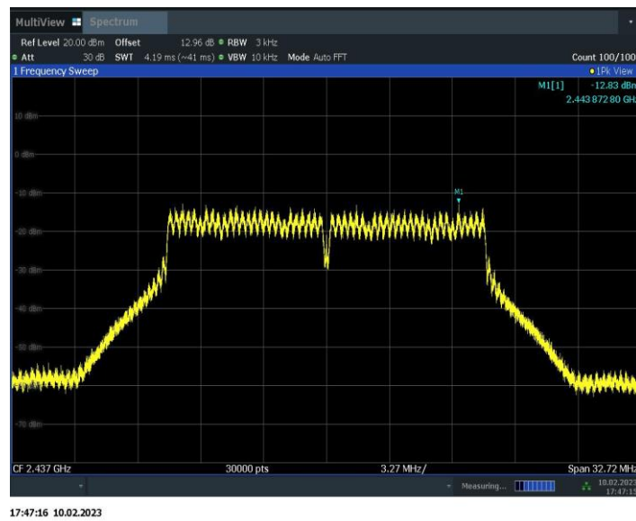
Fig.A.3.5 Power Spectral Density (802.11g, Ch 6)
