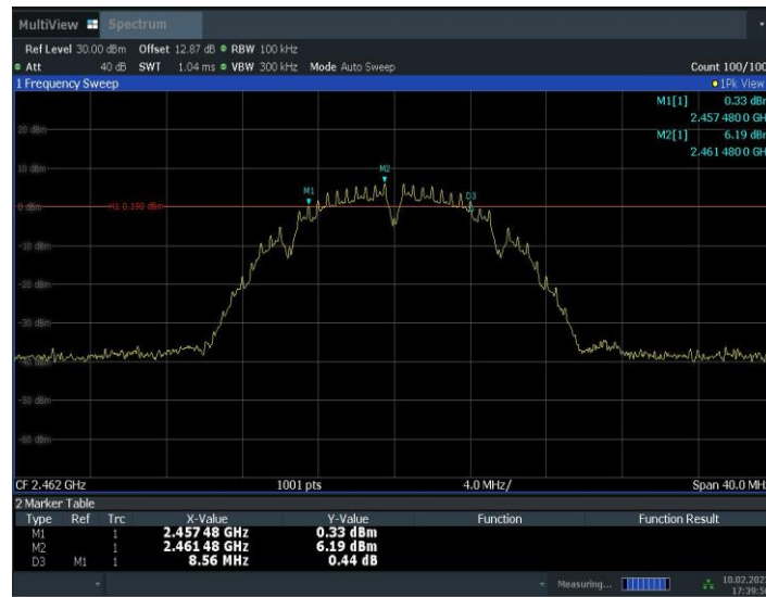
Fig.A.4.3 Occupied 6dB Bandwidth (802.11b, Ch 11)
