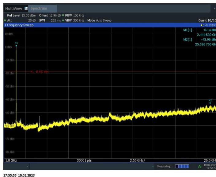
Fig.A.6.1.24 Transmitter Spurious Emission - Conducted (802.11n-HT20, Ch6, 1 GHz-26.5 GHz)
