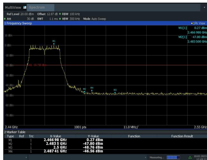
Fig.A.5.4 Band Edges (802.11g, Ch 11)
