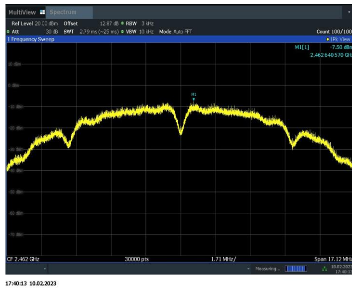
Fig.A.3.3 Power Spectral Density (802.11b, Ch 11)
