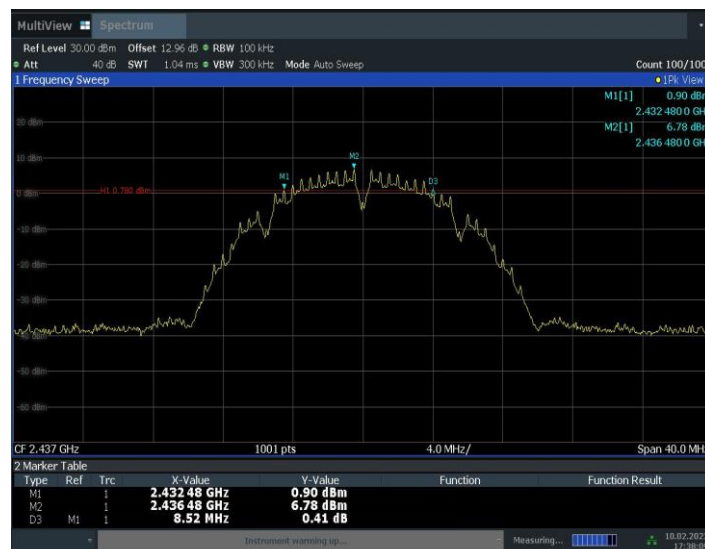
Fig.A.4.2 Occupied 6dB Bandwidth (802.11b, Ch 6)
