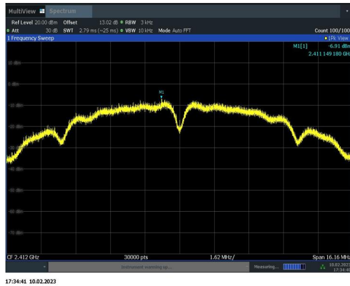
Fig.A.3.1 Power Spectral Density(802.11b,Ch1)
