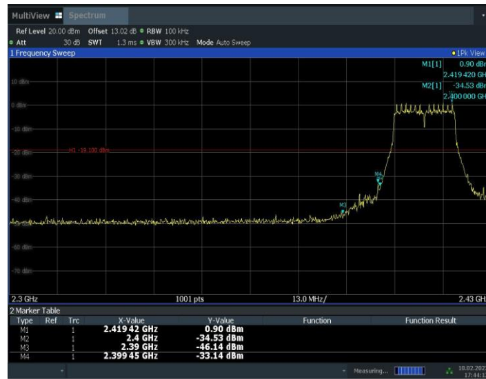
Fig.A.5.3 Band Edges (802.11g, Ch 1)
