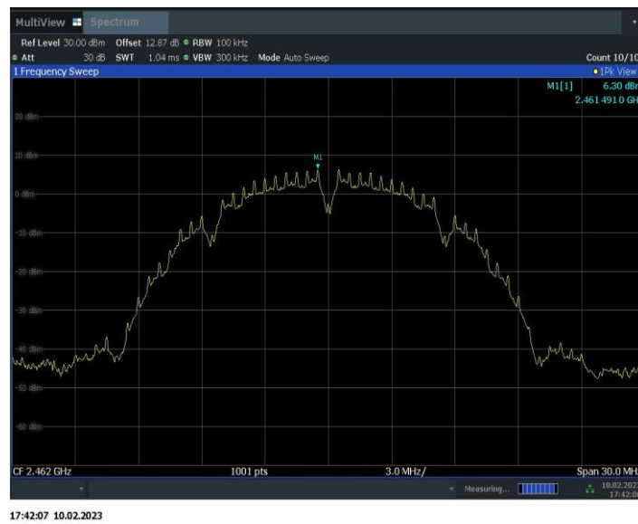
Fig.A.6.1.7 Transmitter Spurious Emission - Conducted (802.11b, Ch11, Center Frequency)
