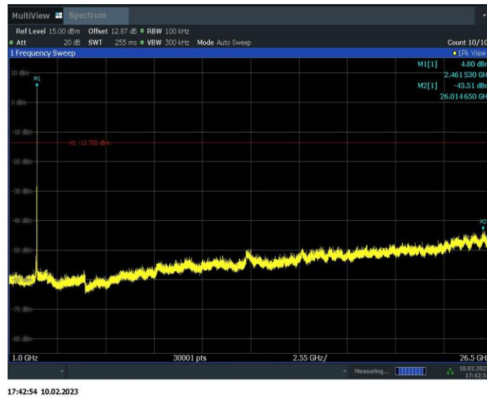
Fig.A.6.1.9 Transmitter Spurious Emission - Conducted (802.11b, Ch11, 1 GHz-26.5 GHz)
