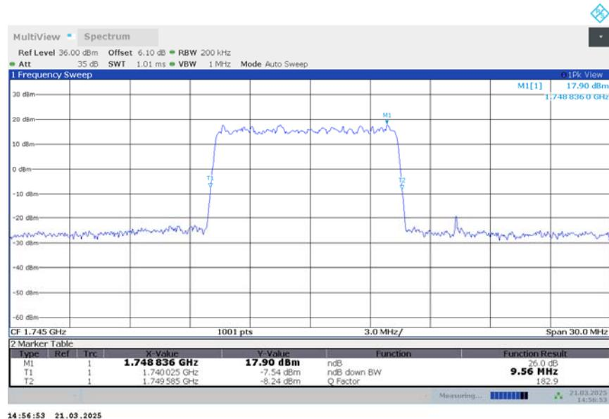
**n66,10MHz Bandwidth,DFT-s-16QAM (-26dBc BW)**
