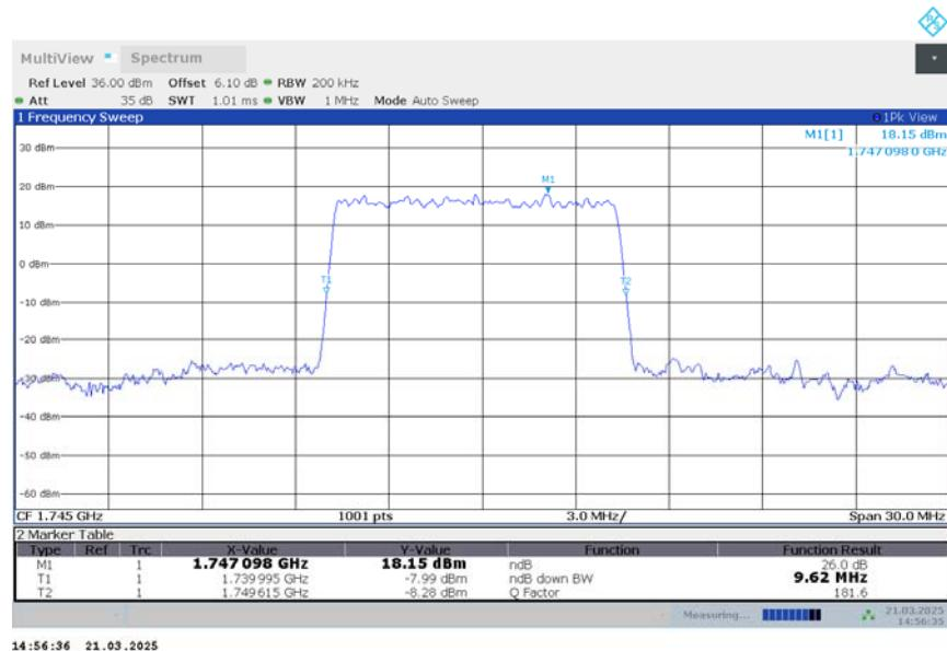
**n66,10MHz Bandwidth,DFT-s-QPSK (-26dBc BW)**
