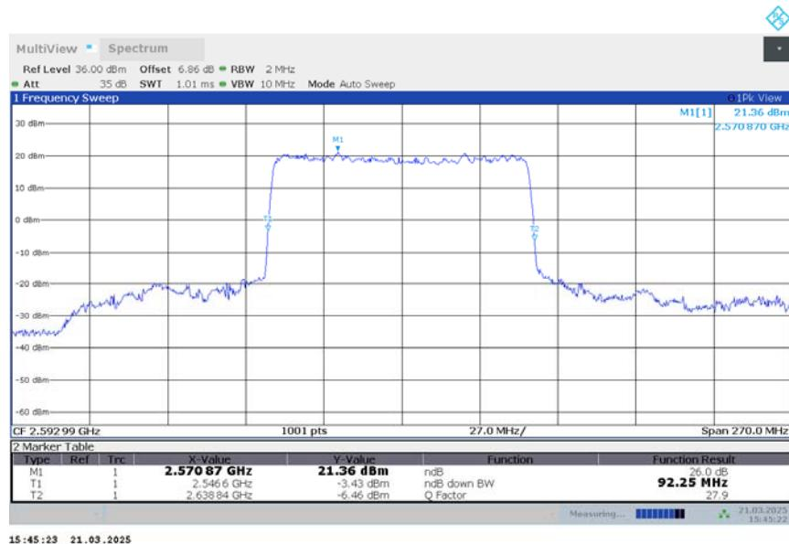
n41,90MHz Bandwidth,DFT-s-QPSK (-26dBc BW)
