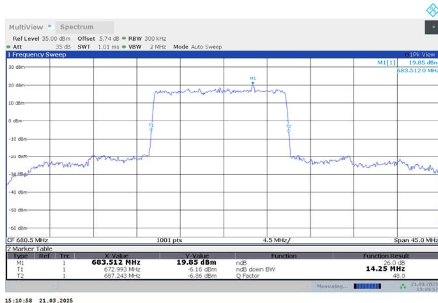
n71,15MHz Bandwidth,DFT-s-QPSK (-26dBc BW)
