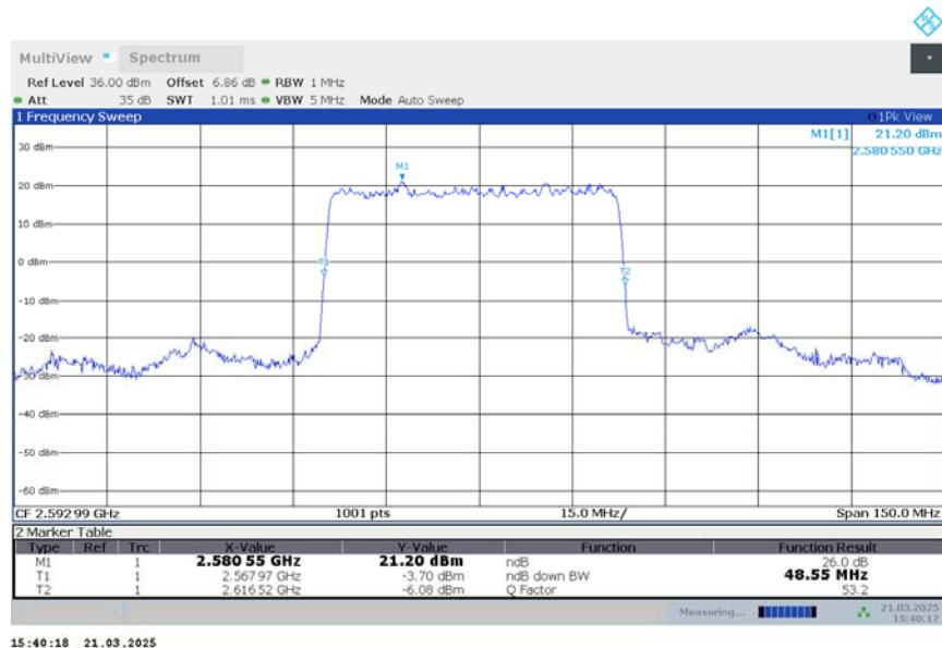
n41,50MHz Bandwidth,DFT-s-QPSK (-26dBc BW)
