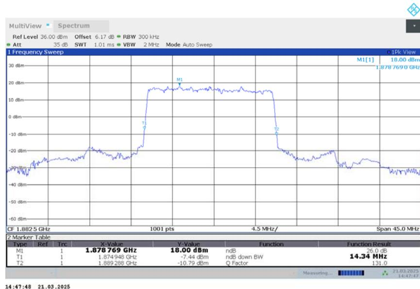
**n25,15MHz Bandwidth,DFT-s-QPSK (-26dBc BW)**
