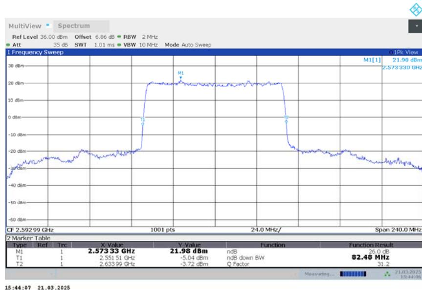
n41,80MHz Bandwidth,DFT-s-QPSK (-26dBc BW)
