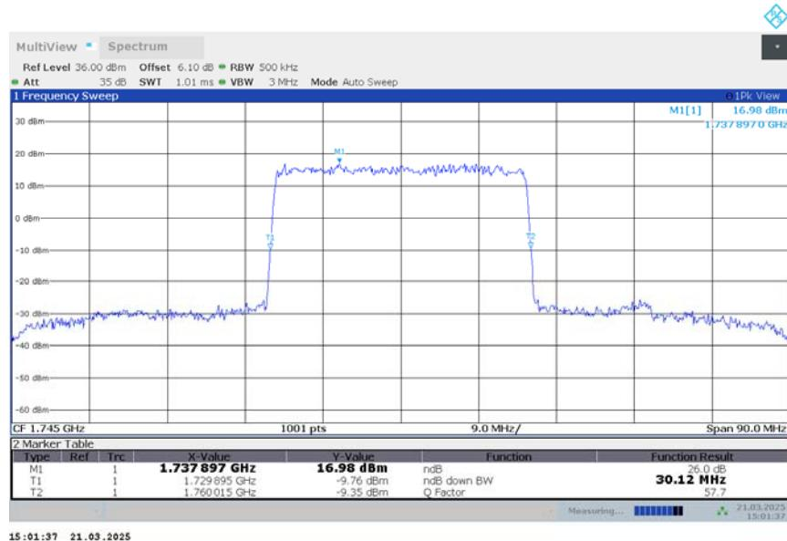
**n66,30MHz Bandwidth,DFT-s-QPSK (-26dBc BW)**
