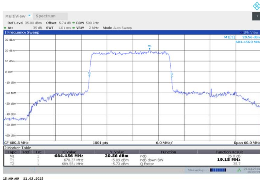
**n71,20MHz Bandwidth,DFT-s-QPSK (-26dBc BW)**
