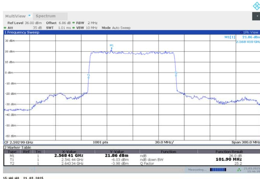
n41,100MHz Bandwidth,DFT-s-QPSK (-26dBc BW)
