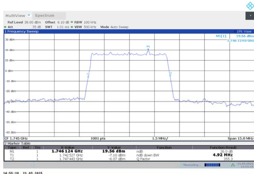
**n66,5MHz Bandwidth,DFT-s-QPSK (-26dBc BW)**
