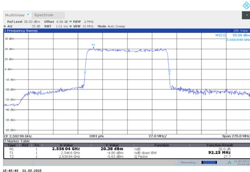
**n41,90MHz Bandwidth,DFT-s-16QAM (-26dBc BW)**
