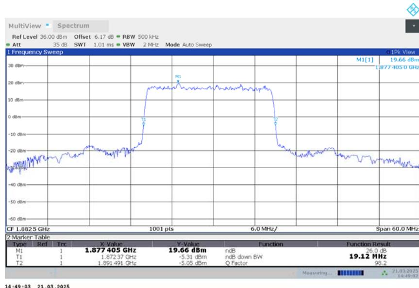
**n25,20MHz Bandwidth,DFT-s-QPSK (-26dBc BW)**
