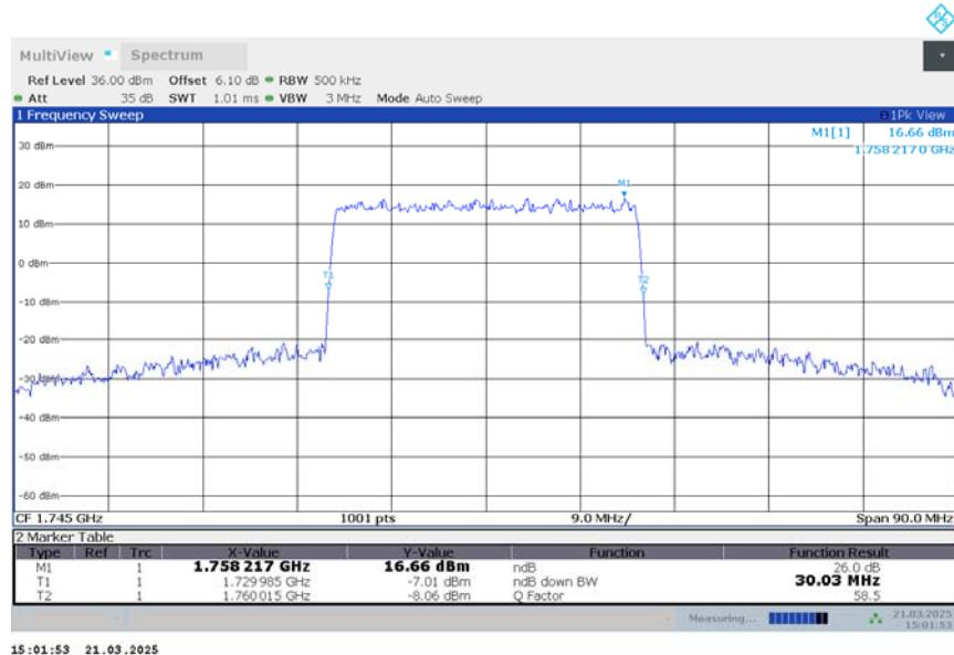
**n66,30MHz Bandwidth,DFT-s-16QAM (-26dBc BW)**
