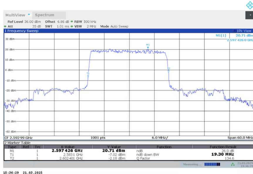
**n41,20MHz Bandwidth,DFT-s-QPSK (-26dBc BW)**
