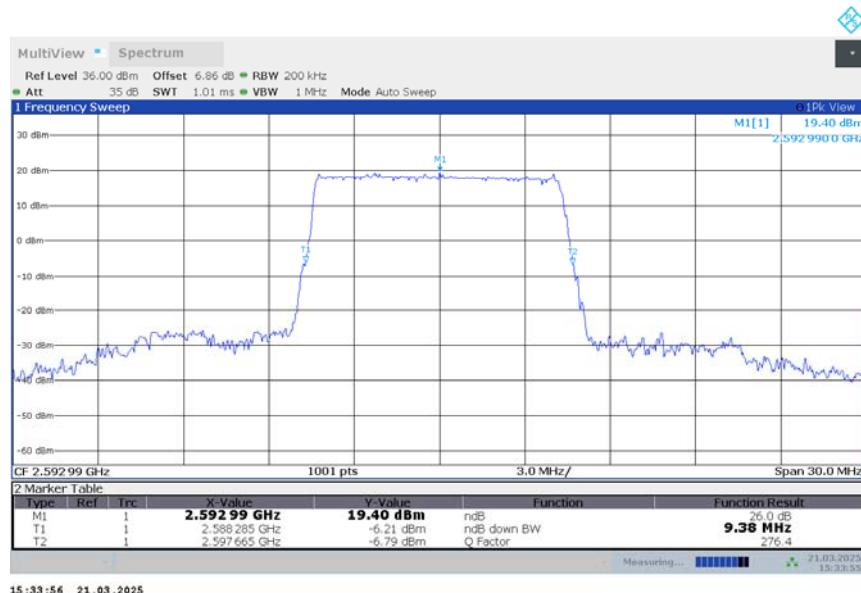
**n41,10MHz Bandwidth,DFT-s-QPSK (-26dBc BW)**
