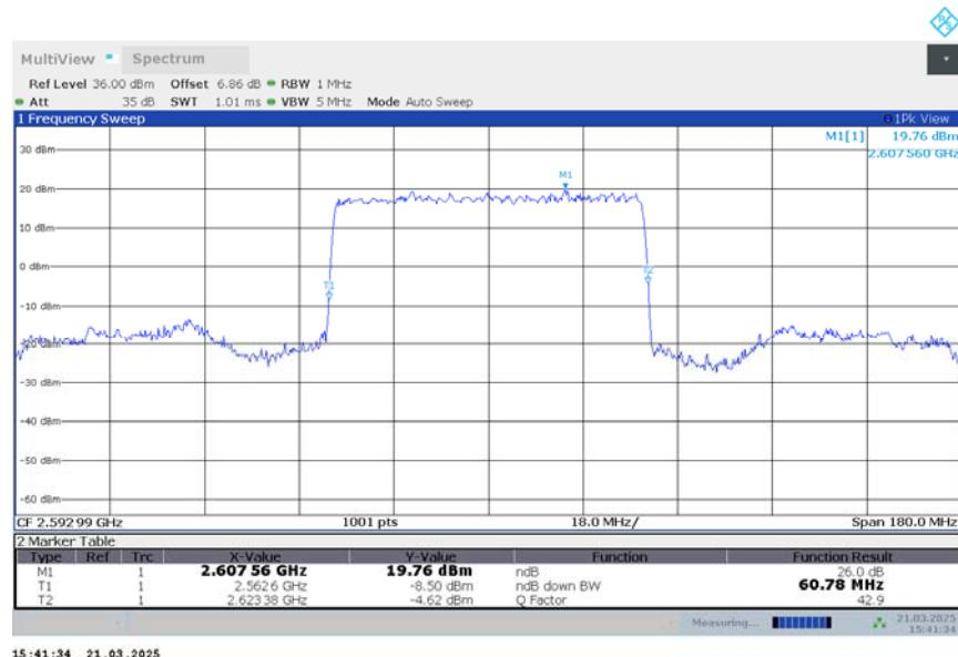
n41,60MHz Bandwidth,DFT-s-QPSK (-26dBc BW)
