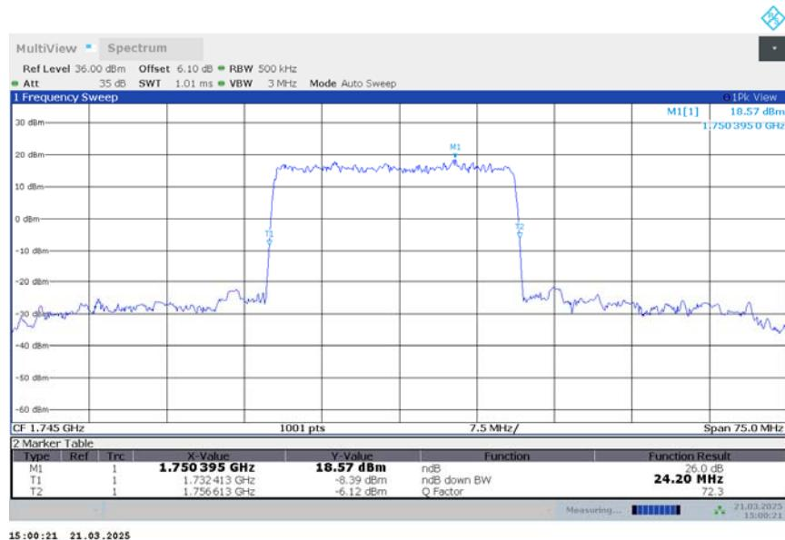
n66,25MHz Bandwidth,DFT-s-QPSK (-26dBc BW)
