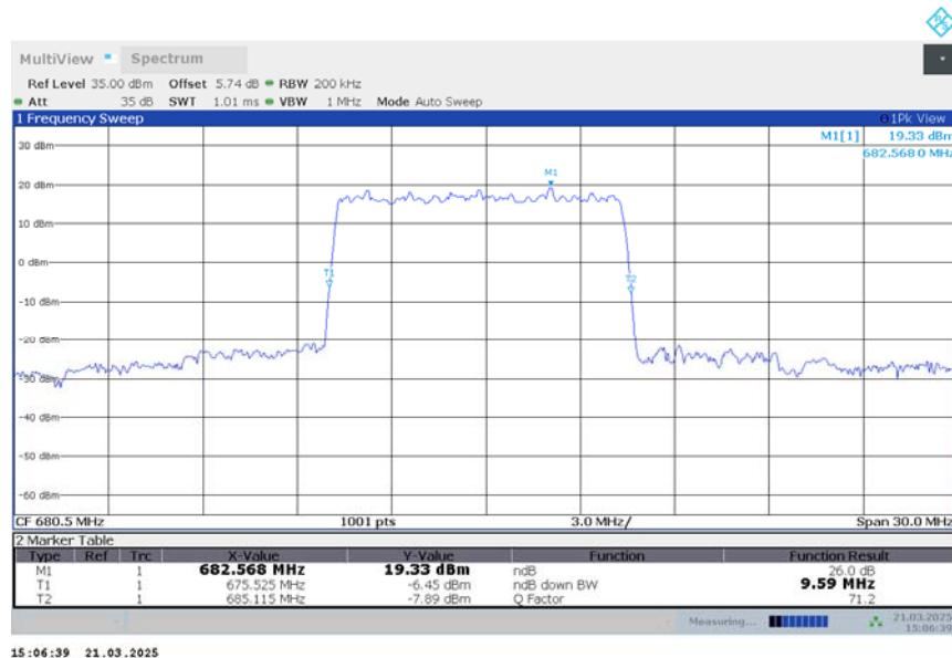
**n71,10MHz Bandwidth,DFT-s-QPSK (-26dBc BW)**
