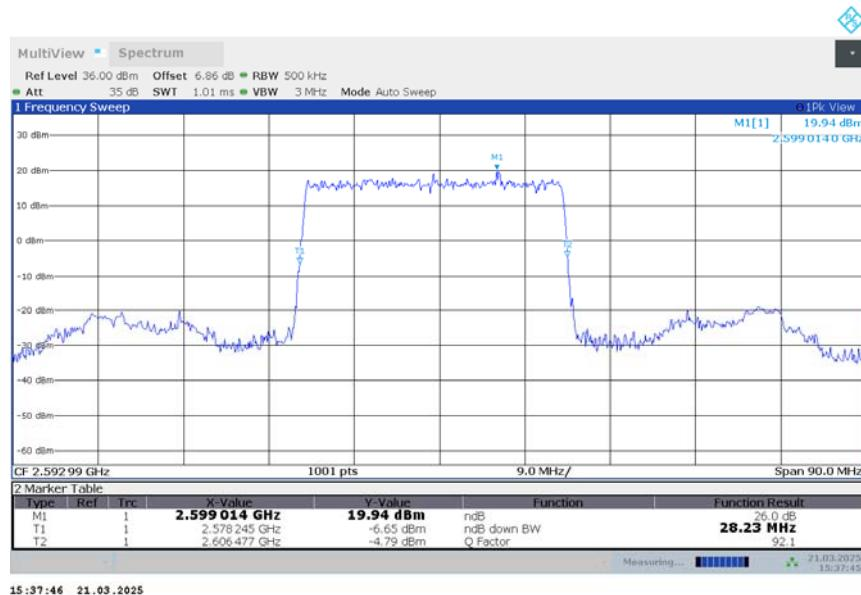
n41,30MHz Bandwidth,DFT-s-QPSK (-26dBc BW)
