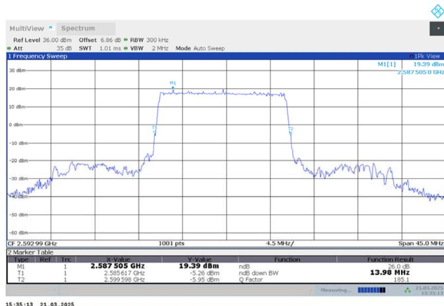
n41,15MHz Bandwidth,DFT-s-QPSK (-26dBc BW)
