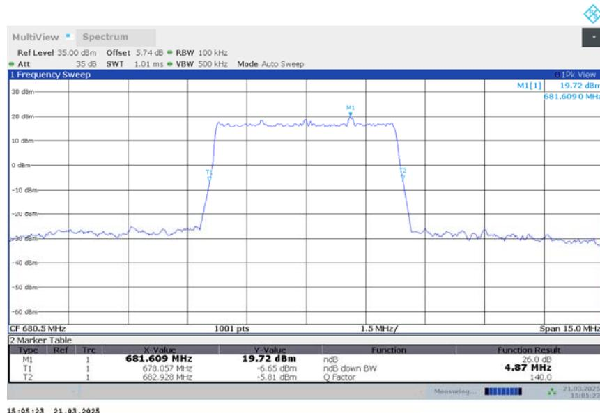
n71,5MHz Bandwidth,DFT-s-QPSK (-26dBc BW)
