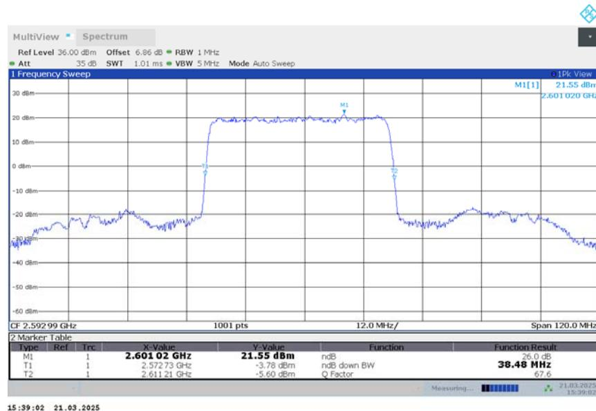
n41,40MHz Bandwidth,DFT-s-QPSK (-26dBc BW)
