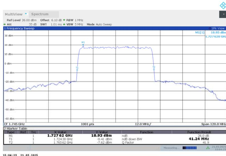
**n66,40MHz Bandwidth,DFT-s-16QAM (-26dBc BW)**
