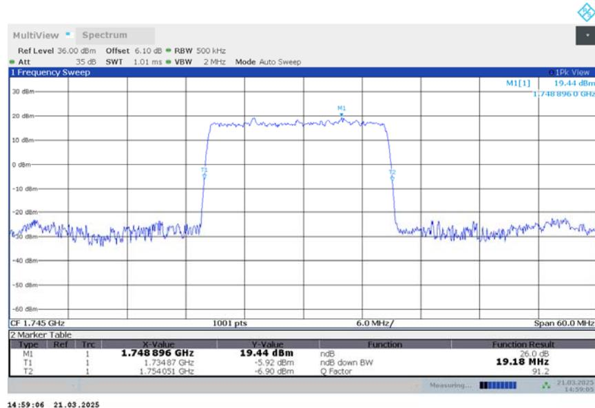
**n66,20MHz Bandwidth,DFT-s-QPSK (-26dBc BW)**
