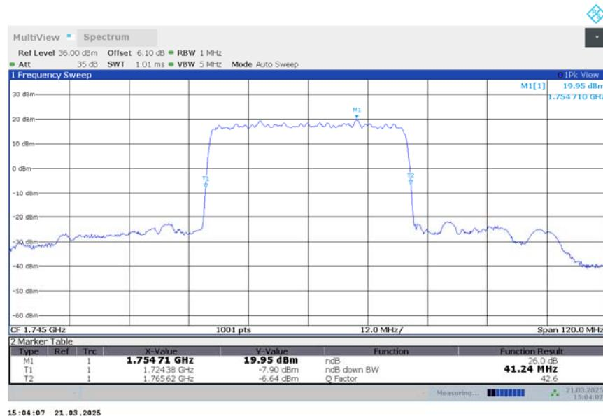
**n66,40MHz Bandwidth,DFT-s-QPSK (-26dBc BW)**
