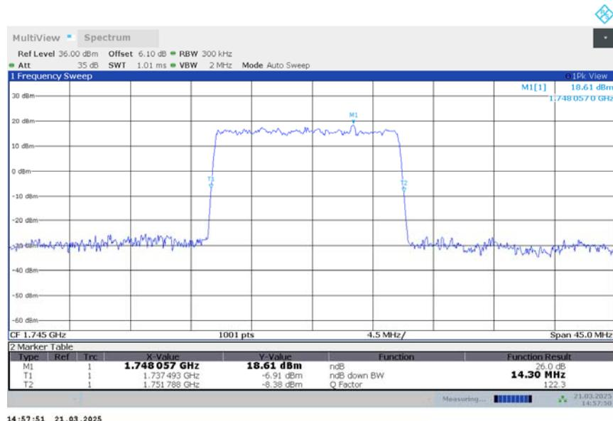
**n66,15MHz Bandwidth,DFT-s-QPSK (-26dBc BW)**
