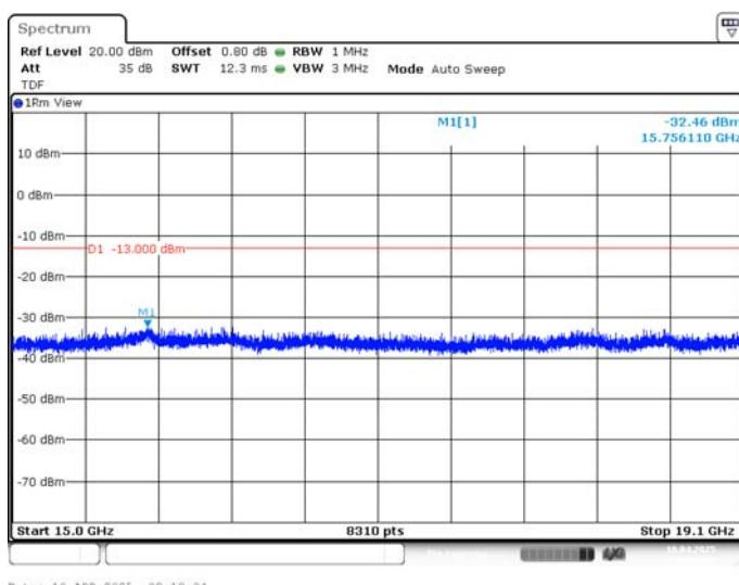
**LTE band 12****NOTE: peak above the limit line is the carrier frequency.**
