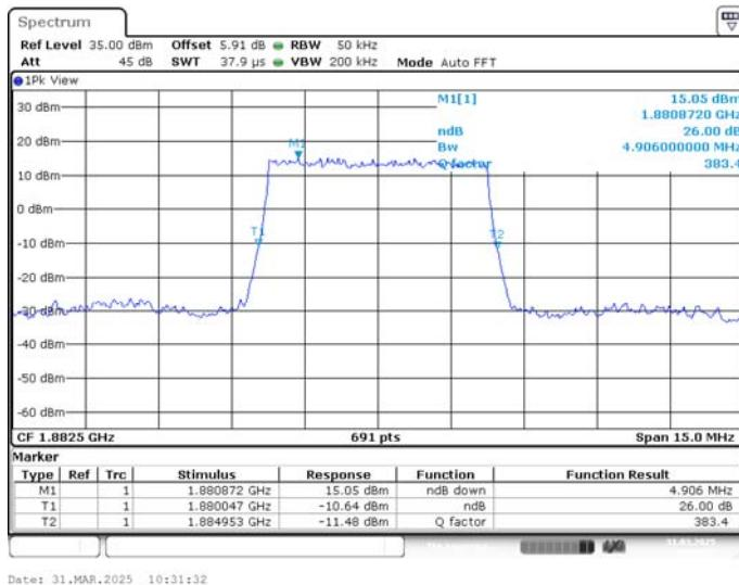
**LTE band 25 , 5MHz Bandwidth,MID,16QAM (-26dBc BW)**
