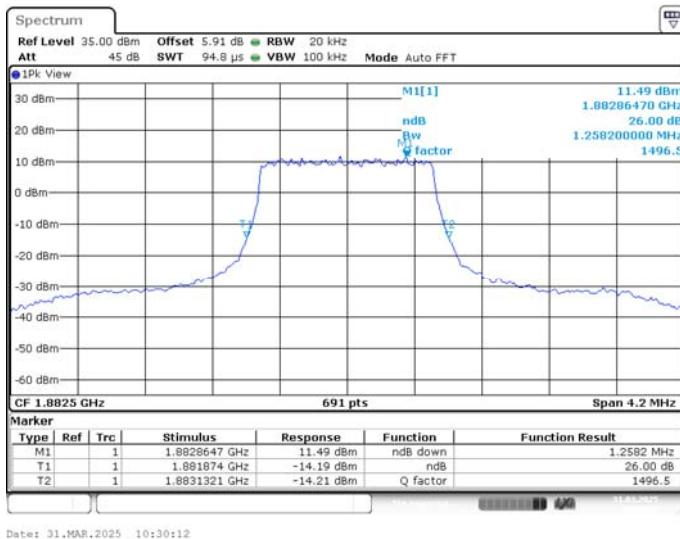
**LTE band 25 , 1.4MHz Bandwidth,MID,16QAM (-26dBc BW)**
