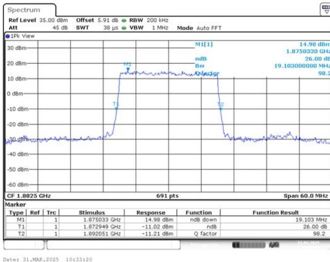
**LTE band 25 , 20MHz Bandwidth,MID,16QAM (-26dBc BW)**
