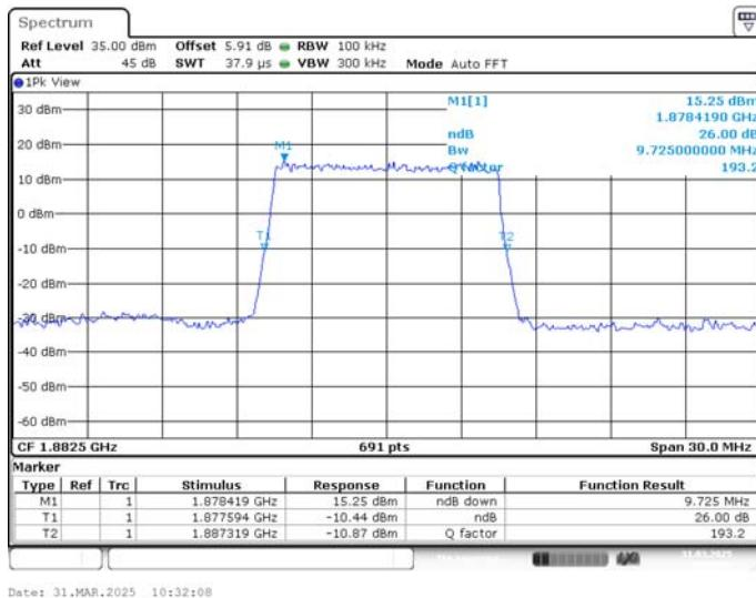
**LTE band 25 , 10MHz Bandwidth,MID,16QAM (-26dBc BW)**
