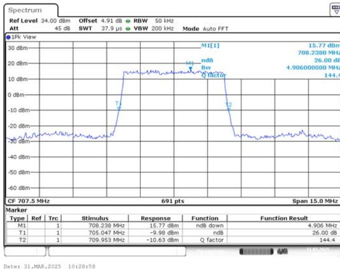
**LTE band 12 , 5MHz Bandwidth,MID,16QAM (-26dBc BW)**
