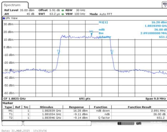
**LTE band 25 , 3MHz Bandwidth,MID,16QAM (-26dBc BW)**
