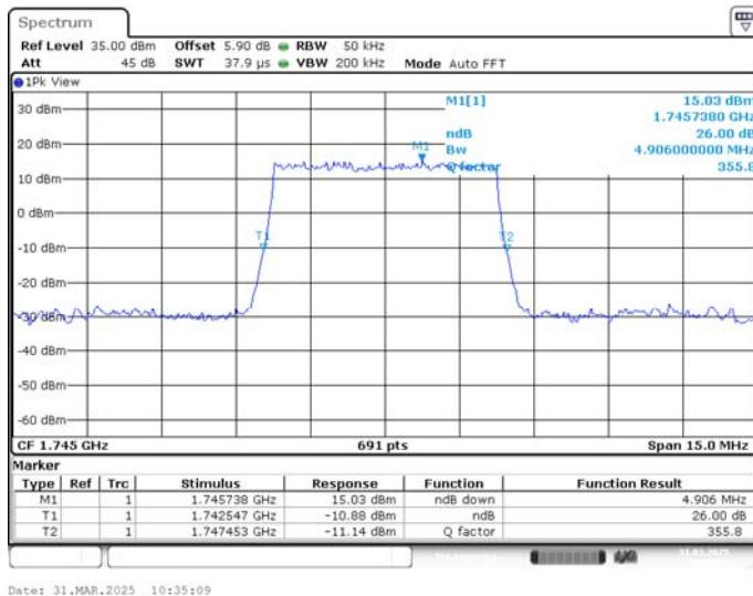
**LTE band 66 , 5MHz Bandwidth,MID,16QAM (-26dBc BW)**
