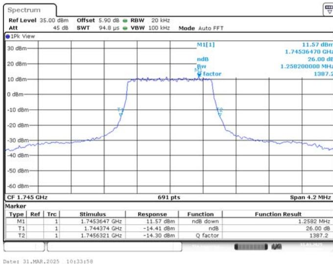
**LTE band 66 , 1.4MHz Bandwidth,MID,16QAM (-26dBc BW)**
