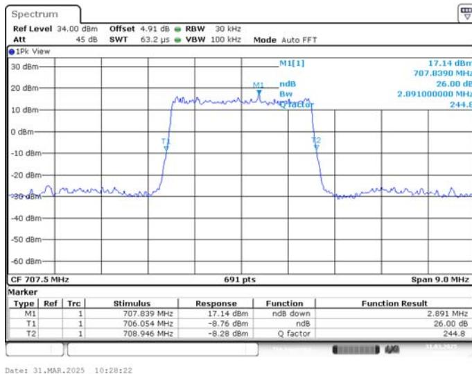
**LTE band 12 , 3MHz Bandwidth,MID,16QAM (-26dBc BW)**
