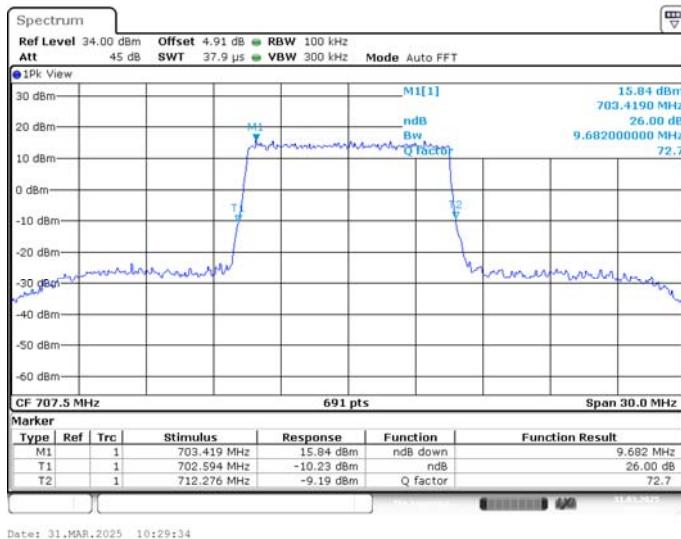
**LTE band 12 , 10MHz Bandwidth,MID,16QAM (-26dBc BW)**
