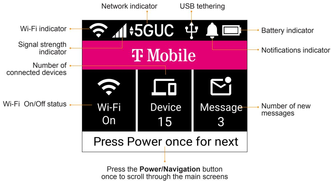
Note: The display will timeout after 30 seconds of inactivity to save power. Press the **Power/Navigation** button one time to wake the screen. This default setting can be adjusted on the WebUI (<http://mifimanager> or <http://192.168.0.1>) under **System > Device > Turn off screen**.
