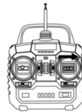
When the aileron control lever of the transmitter is pushed rightward, the aircraft will tilt rightward.
