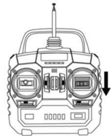
When the lifting control lever of the transmitter is pulled down, the rudder of the horizontal tail will move up and the aircraft will ascend.
