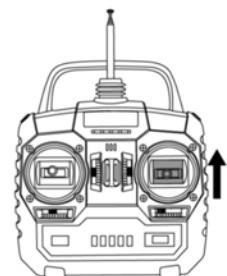
When the lifting control lever of the transmitter is pushed up, the rudder of the horizontal tail will move down and the aircraft will descend.
