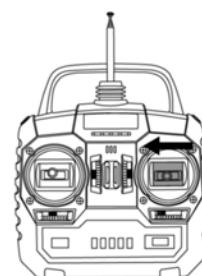
When the aileron control lever of the transmitter is pushed leftward, the aircraft will tilt leftward.
