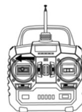
When the direction control lever of the transmitter is pushed leftward, the aircraft will turn left.
