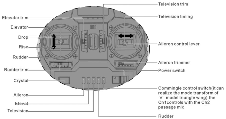
Before starting the aircraft test flight, please carefully check and make sure the transmitter and the server work normally. Then turn on the transmitter before connecting the battery to the receiver (the opposite for turning off).
