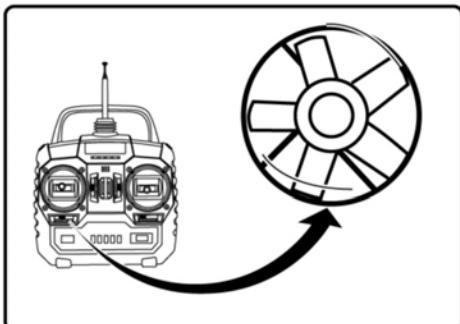
Put 8 X AA alkaline batteries into the transmitter and turn on the power switch.
