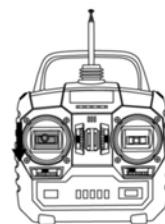
When the lifting control lever of the transmitter is pulled down, the rudder of the horizontal tail will move up and the aircraft will ascend.
