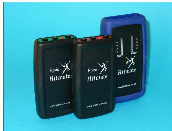
An Epee Hitmate set comprises three units: A pair of Hitmate units (one Red, one Green) and a Hitmate Floor Console. All three should show the same number on the edge. Hitmate uses a single radio frequency and the numbers allow units to recognise each other. This also allows many Hitmates to be used within the same venue.
