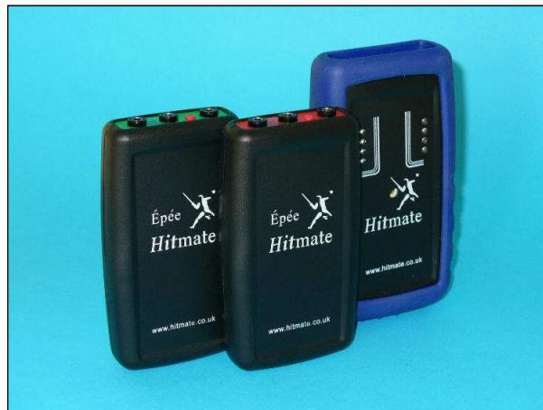
An Epee Hitmate set comprises three units: A pair of Hitmate units (one Red, one Green) and a Hitmate Floor Console. All three should show the same number on the edge. Hitmate uses a single radio frequency and the numbers allow units to recognise each other. This also allows many Hitmates to be used within the same venue.
