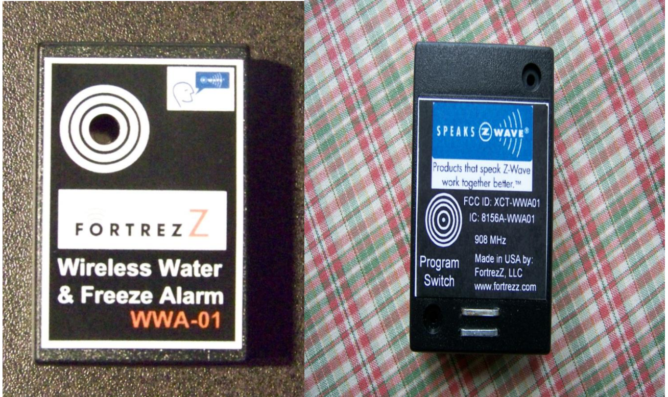
Figure 1: The Fortrezz WWA-01 Wireless Water and Freeze Alarm, Front View (Left) and Back View (Right)
