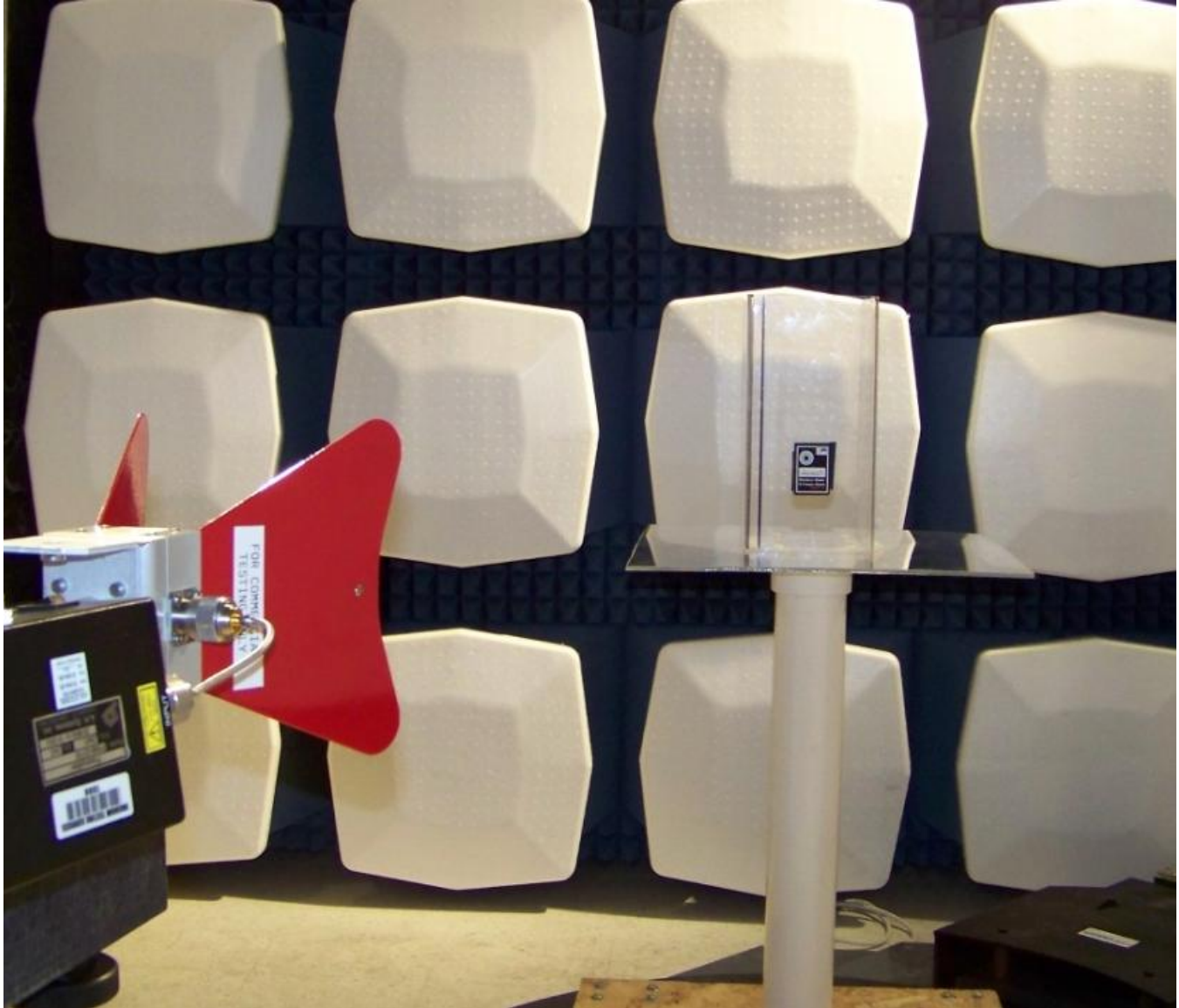
Figure 6: EUT on Test Pedestal; Emission Testing Above 1 GHz, at 1m Separation Distance
