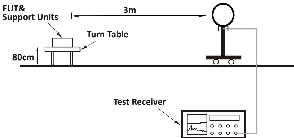
**For Radiated emission 30MHz to 1GHz:**
