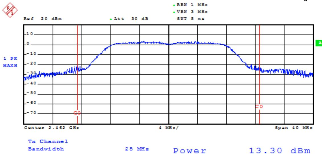
**Low Channel for Antenna B****Test mode: 802.11b**
