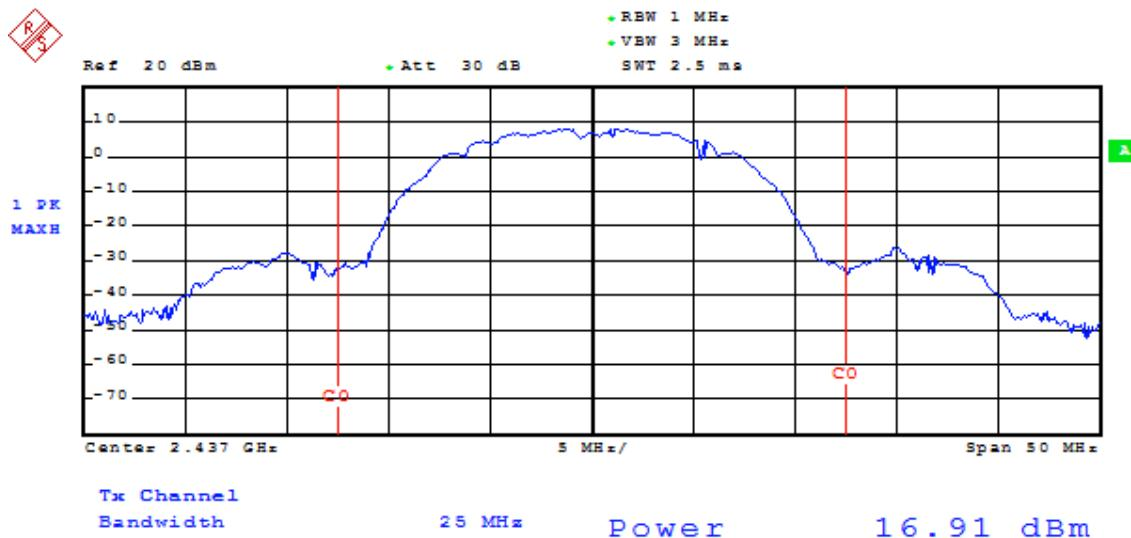
**High Channel for Antenna A****Test mode: 802.11b**
