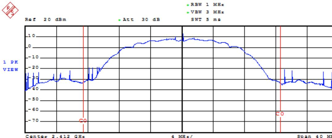
**Tx Channel** Bandwidth 25 MHz Power 16.93 dBm
