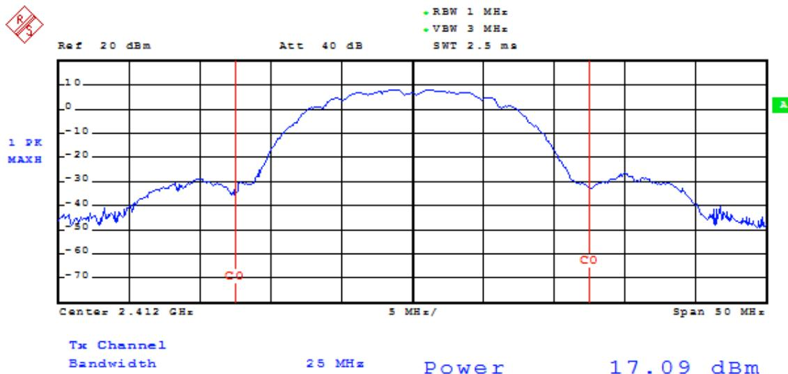
**Mid Channel for Antenna A****Test mode: 802.11b**
