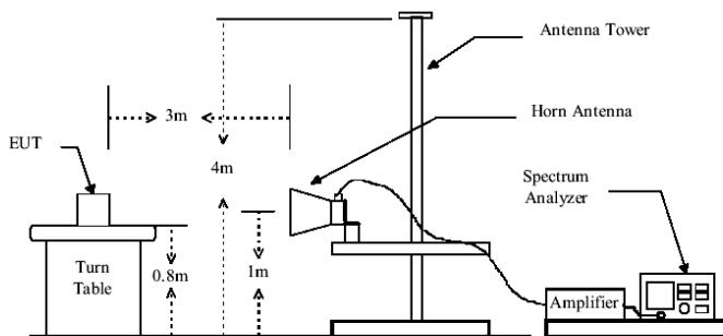
The field strength is calculated by adding the Antenna Factor, Preamplifier Factor & Cable Factor. The basic equation with a sample calculation is as follows:
