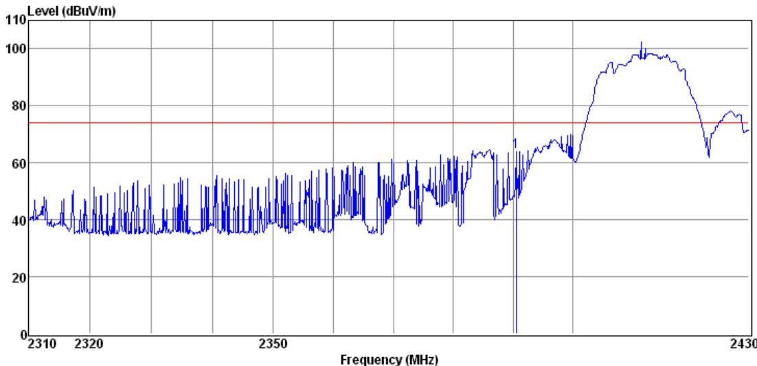
**802.11b Low Channel for Antenna A****Horizontal, Average Detector:**
