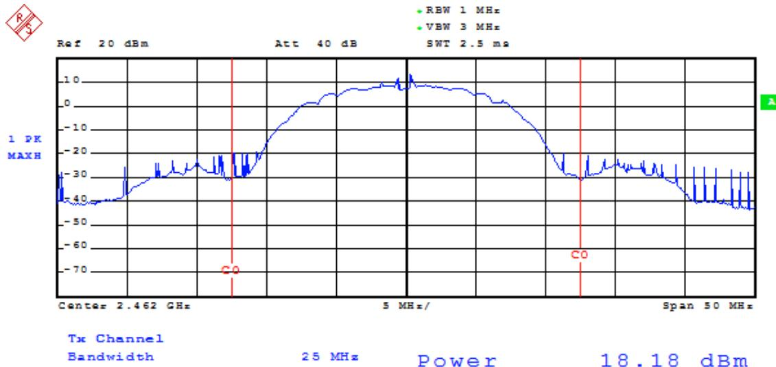
**Low Channel for Antenna A****Test mode: 802.11g**
