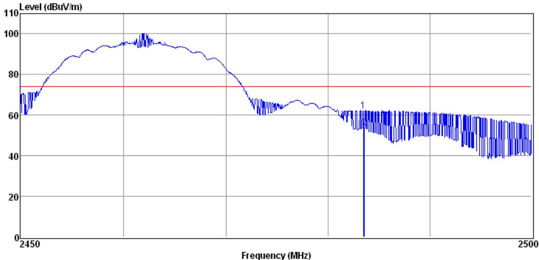
**802.11b High Channel for Antenna B****Horizontal, Average Detector:**
