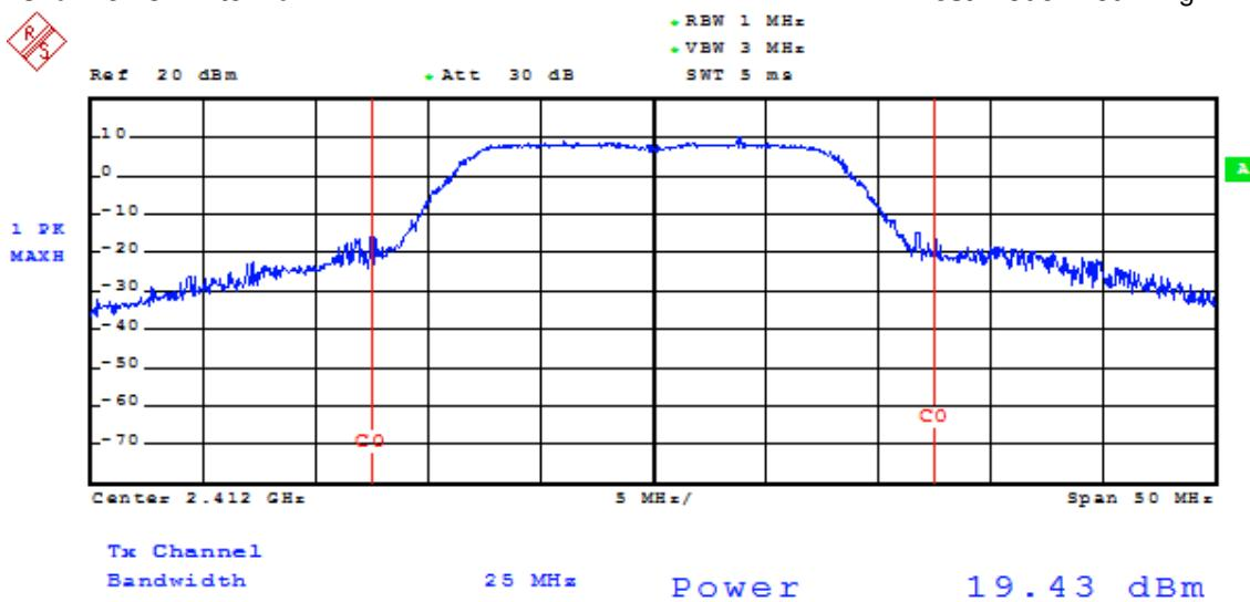
**Mid Channel for Antenna B****Test mode: 802.11g**
