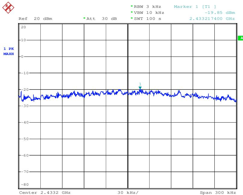
**High Channel for Antenna A****Test mode: 802.11g**
