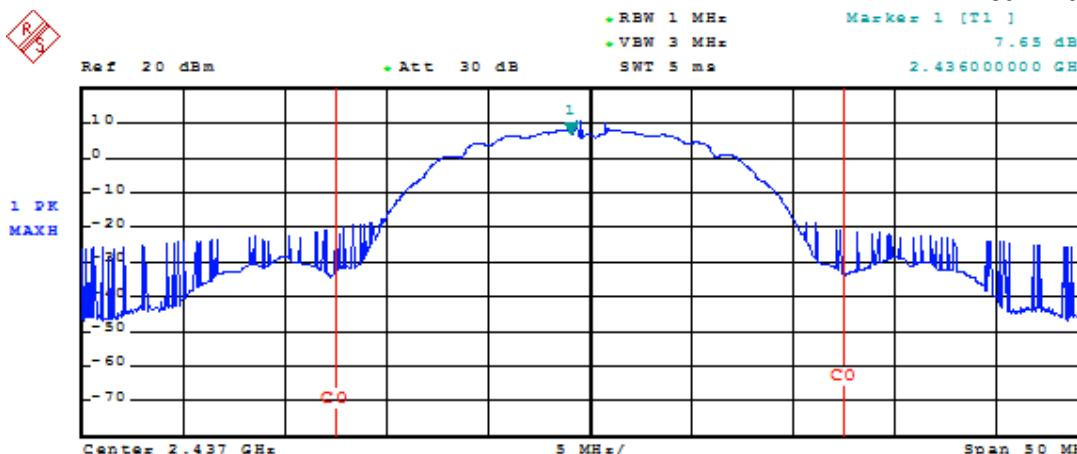
**Tx Channel** Bandwidth 25 MHz Power 16.92 dBm
