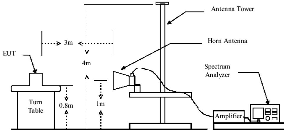
Low noise amplifier was used below 1GHz, High pass Filter was used above 1GHz.
