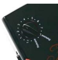
Synchronization is available when Firefox R1 and Firefox P1 are set at the same channel. Basically, 1 1:1 channel, wireless release channel, 7 normal channels are provided. (1 channel is used as Reset channel in Firefox P1)
