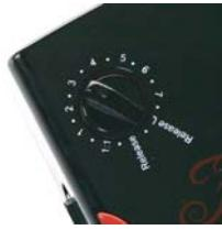
When it is set at wireless release Lock channel among channels, shutter cover of camera (Bulb mode of camera) is opened by pushing release button once and closed by pushing it twice.
