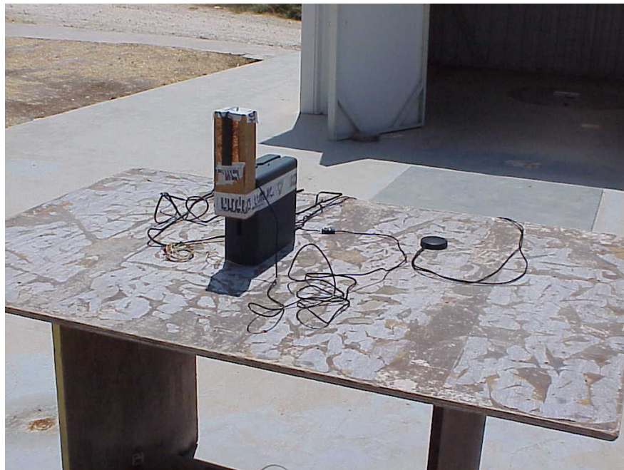
Photo 3. Spurious emissions test setup. Typically installation of external antenna on metal surface.
