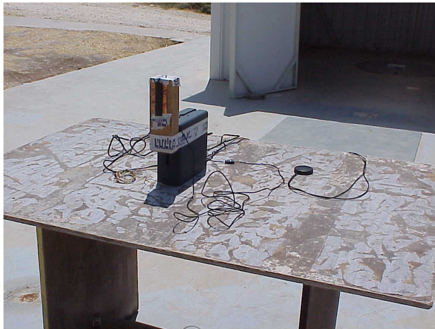
Photo 3. Antenna typical installation on metal surface. Typically installation of external antenna on metal surface.
