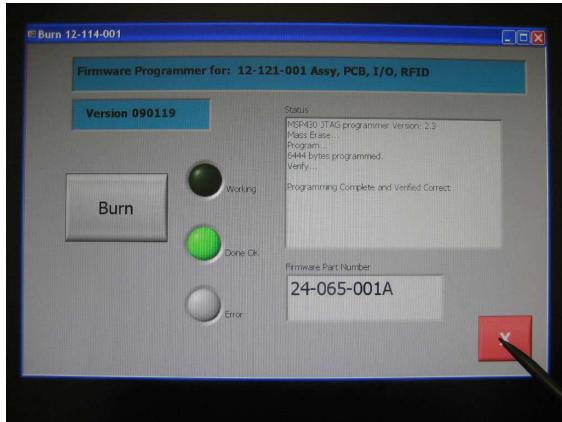
When all PCB Assemblies are programmed, close the program by tapping once on the red button with an “X” in the lower right corner of the program screen.
