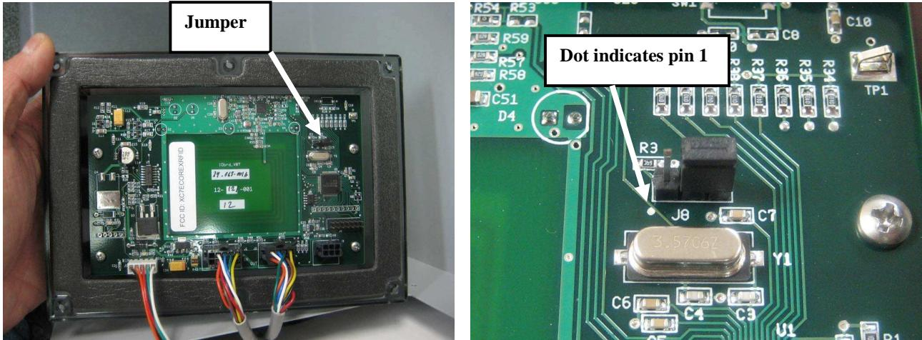
Verify Connector, Jumper Shorting, Gold is on pins 2 and 3 of Jumper J8 on each Assembly, Window/PCB RFID/Software as shown.
