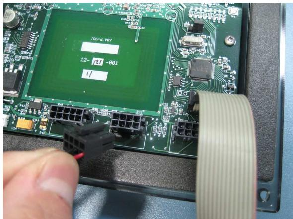
Using 12 volt power supply insert 8 pin connector on I/O power cable into 8 pin receptacle on PCB Assembly.
