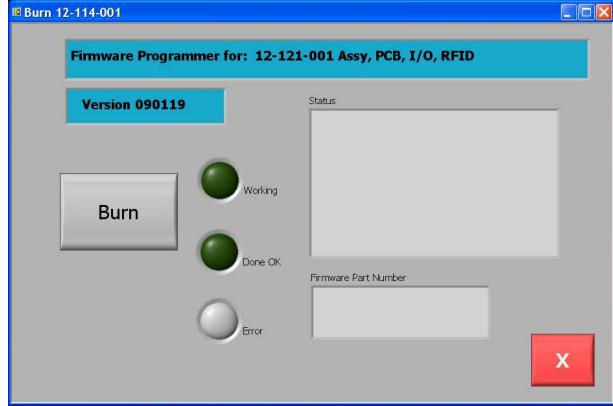
Double click on the icon named “12-121-001 Assy, PCB,I/O RFID” to start the firmware upload program.
