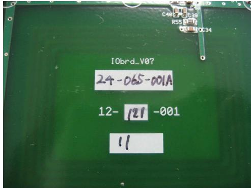
Write Firmware Part Number info using permanent marker on white label area of PCB. Also record the Firmware Part Number Info on the traveler.
