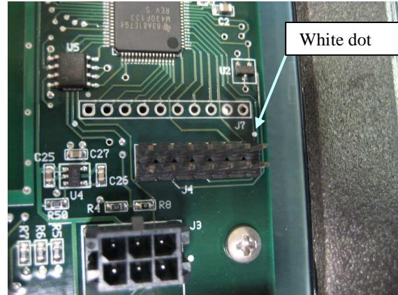
At the board programming station plug the 14 pin connector on Texas Instruments MSP430 USB-Debug-Interface into receptacle J4 on Assembly, Window/PCB RFID/Software. Red wire on 14 pin ribbon cable indicates pin one on connector and should be aligned with white dot indicated on PCB.
