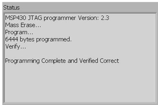
When upload is complete and successful the “Done OK” status indicator will illuminate green and the status screen will read “Programming Complete and Verified Correct”.
