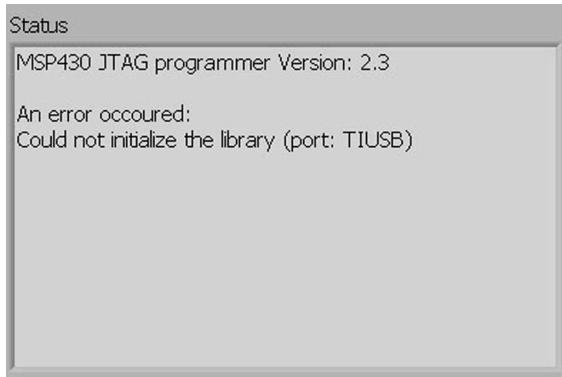
If the error message is “Could not initialize the library (port: TIUSB)”, this indicates that the MSP430’s USB cable is not connected properly. Check USB cable connection to the MSP430 and to the PC computer.
