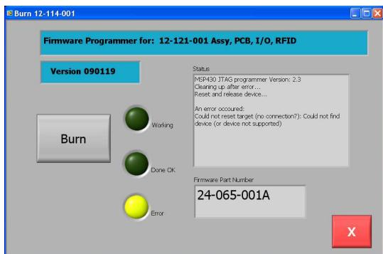
If the yellow indicator comes on during firmware burn a fault has occurred. Troubleshoot by reading the error message in the “Status” box as follows.
