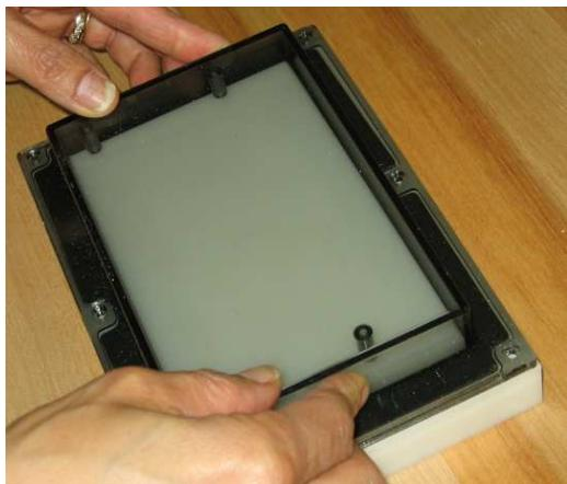
1.4 Secure the Gasket, Level Sensor Window (21-516-001) onto the flange relief by applying even uniform pressure with thumbs along the sealing surface of the gasket.
