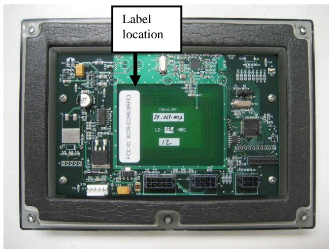
Remove label 33-100-001 from its backing paper and apply label to location as shown. Do not allow label to cover any printing, writing, electrical components or electrical traces.
