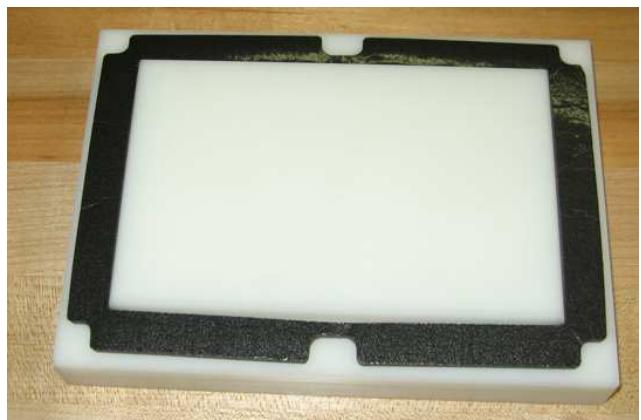
1.3 Place Gasket, Level Sensor Window (21-516-001) onto the Gasket Level Sensor Fixture (T1-011-001). Press down firmly on edges of window and then remove from fixture.
