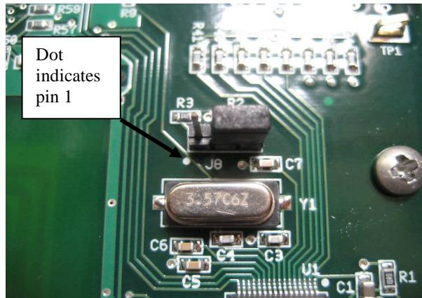
Apply Connector, Jumper Shorting, Gold to pins 2 and 3 of Jumper J8 on each PCB assembly as shown.
