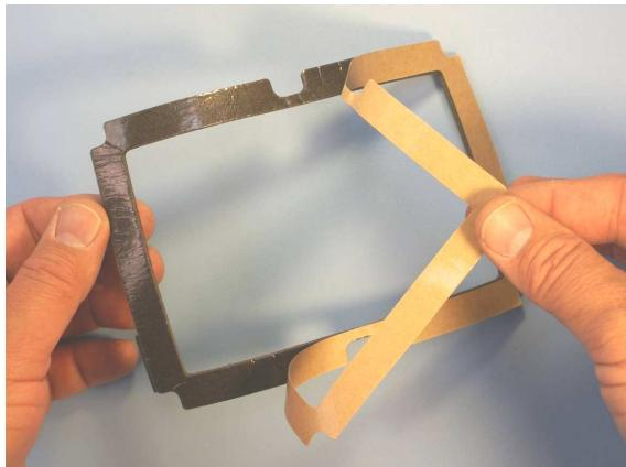
1.2 Carefully align and place the Gasket, Level Sensor Window (21-516-001) adhesive side up on the Gasket Level Sensor Fixture (T1-011-001) .
