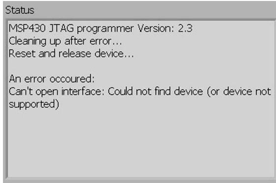
If the error message is “Can’t open interface: Could not find device (or device not supported)”, this indicates that the MSP430 is not connected properly to the PCB. Check the cable connecting the MSP430 to the PCB.
