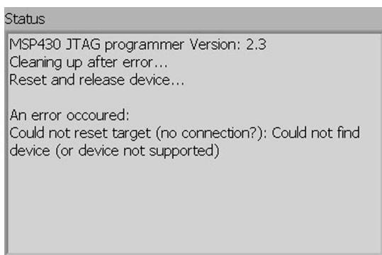
If the error message is “Could not reset target (no connection?): Could not find device (or device not supported)”, this indicates there is no power to the PCB Assembly. Check all power connections.
